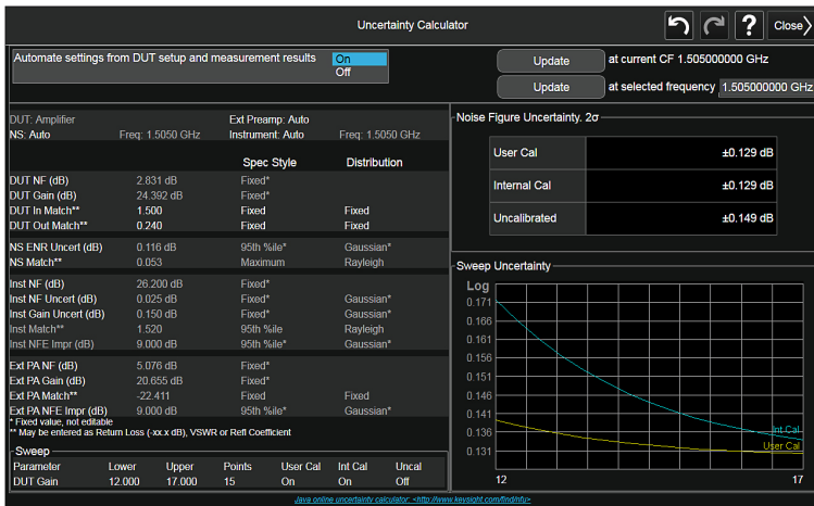
Figure 5-2 X-Series NFA noise figure analyzers and X-Series signal analyzers with noise figure measurement application have a built-in uncertainty calculator with graphical results that can auto-populate instrument, preamplifier and noise source parameters.
