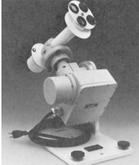
Figure 2.2.3 An Eppley NIP on an altazimuth tracking mount. Courtesy of The Eppley Laboratory.
