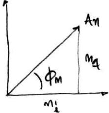
$$m(t) = \underbrace{A_m(t)}_{\text{envolvente}} \cos(\omega t + \underbrace{\phi_m(t)}_{\text{fase}})$$
