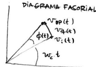
$$v_{pp}(t) = v_i(t) \cos(w_c t) + v_q(t) \cos(w_c t + \frac{\pi}{2}) =$$
