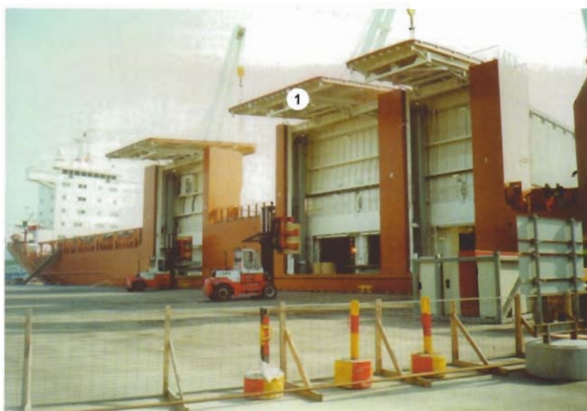
Ship with three side-doors
