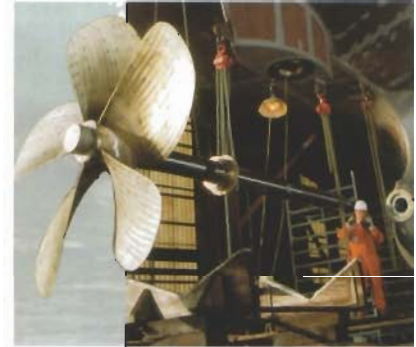
Installation of a fixed right-handed propeller with shaft
