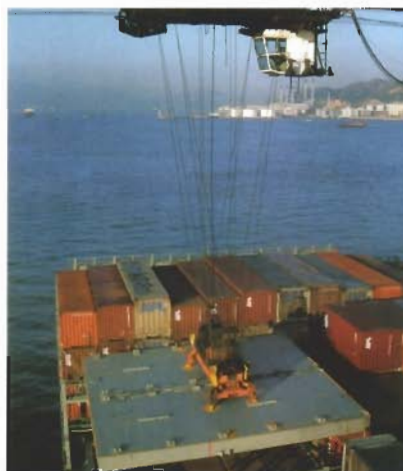
Moving a pontoon hatch with a container crane
