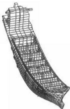
Ship in a trough, sagging
