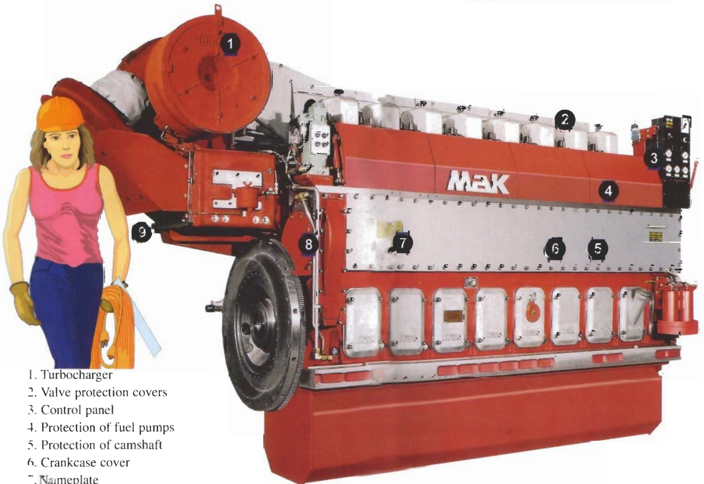
Medium-speed engine, 8 cylinders in line
