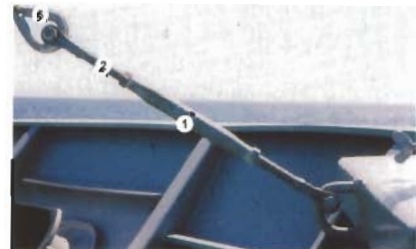
Bottle screw to tighten the foremast stay
