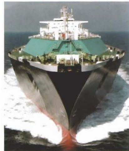
LNG-tanker with a well-designed bulb
