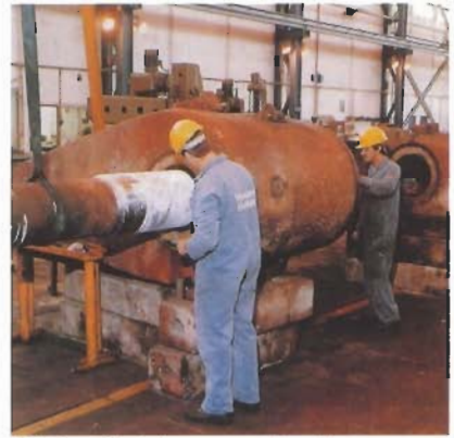
Fitting of pintles to new bushings
