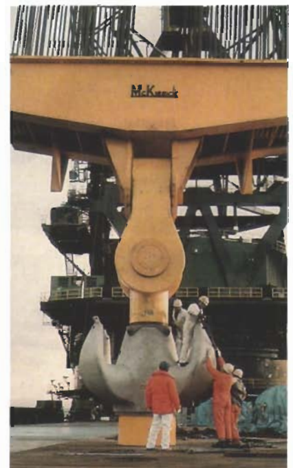
Spreader with hook, SWL 6000 tons
