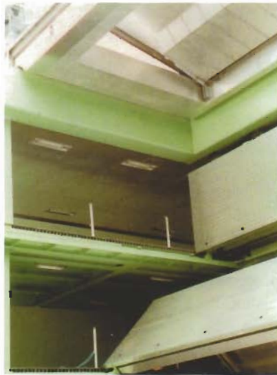
Tweendecks with folding hatches on a reefer.
