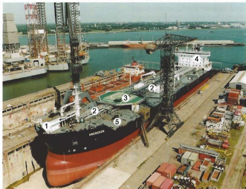
Shuttle tanker in dry dock
