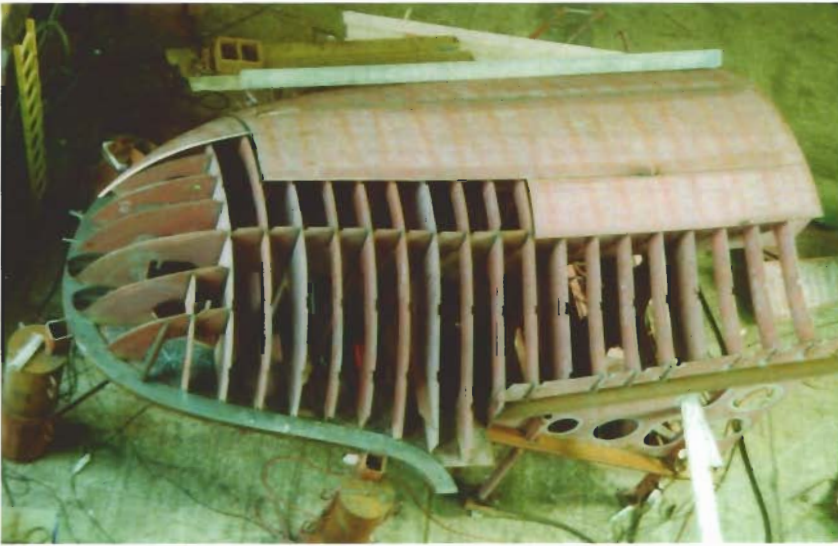
Fitting of the shell plating
