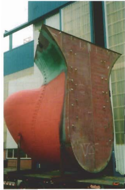
Forepeak, ready to be installed
