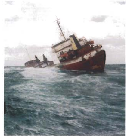
A ship with heel in an unstable situation.
