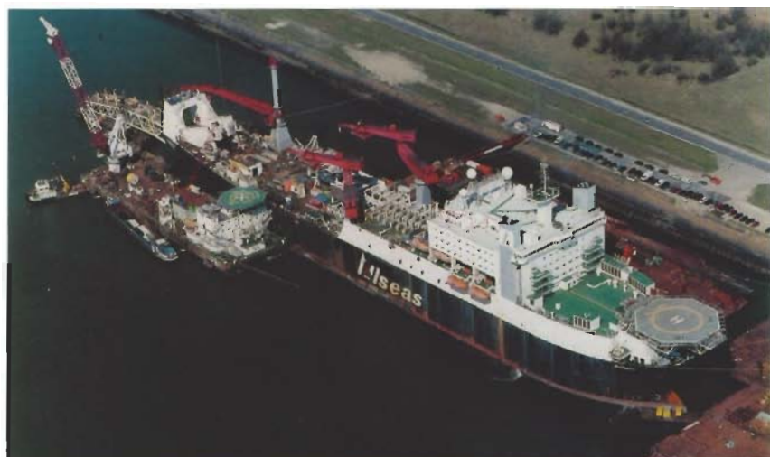
S-lay pipelaying vessel with crane barge alongside
