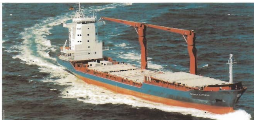
Container feeder with revolving deck cranes
