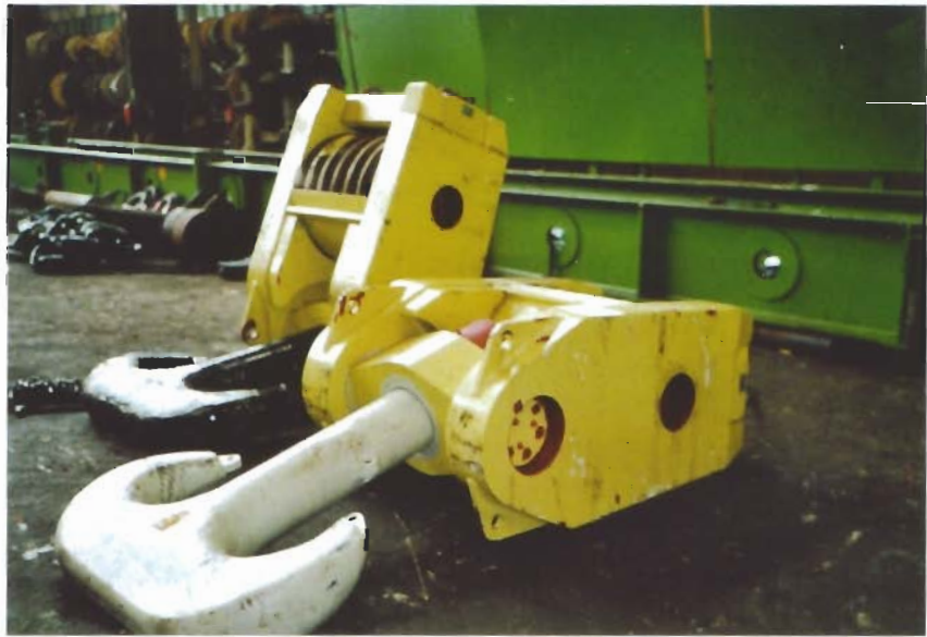
Blocks with rams horns of heavy cargo gear (400 tons SWL)
