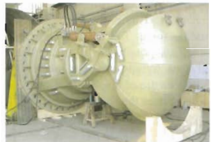
Waterjet with reversing bucket
