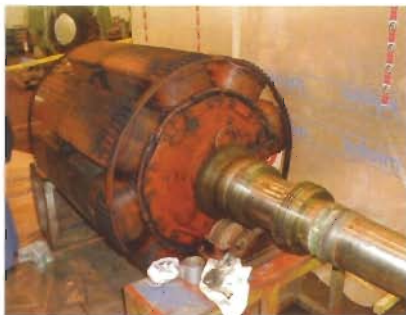
A generator rotor
