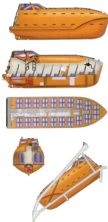
Different views of a free-fall lifeboat
