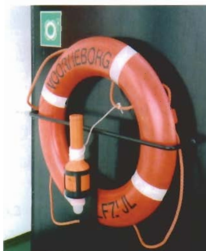
Life buoy with light and marking
