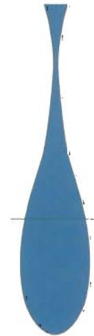
Top view of a fish tail rudder
