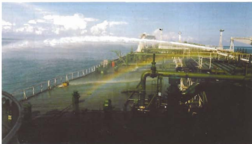
Testing the foam pump on a tanker
