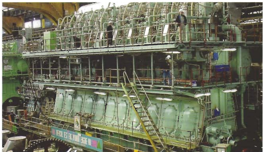
Low-speed engine for large container-ship.
