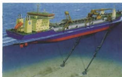
Trailer hopper suction dredger length = 167 meter breadth = 31 meter carrying capacity = 30000 ton
