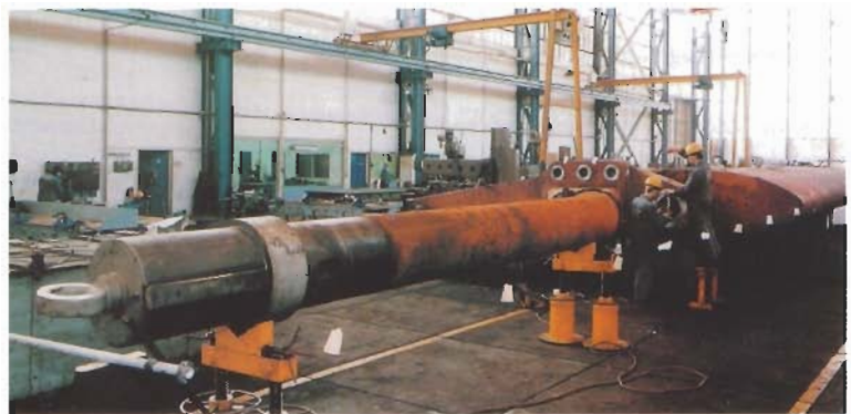
Alignment of rudder and stock in shop
