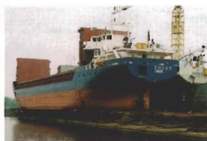
Ship on a patent slip
