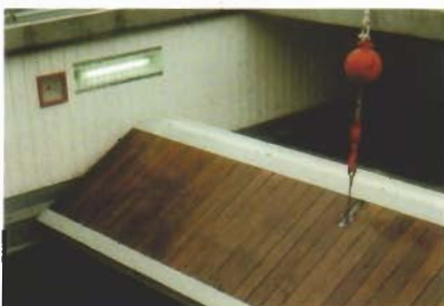
A ship's crane opens a folding hatch
