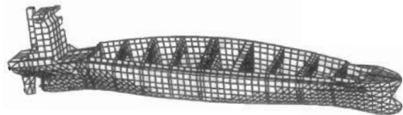
Waves coming in from starboard at an angle, torsion
