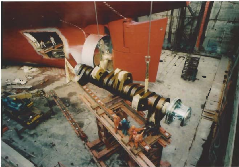
Exchange of crank shaft
