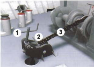
Chain stopper with tensioner
