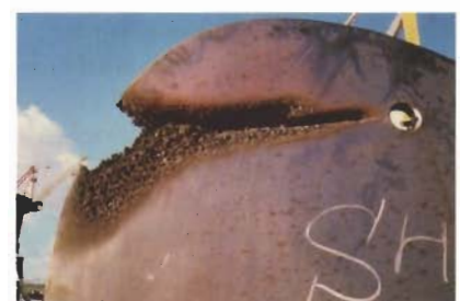
Cavitation damage on a rudder blade due to missing plug.
