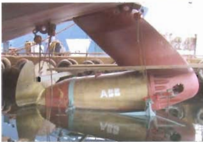
Attaching the azipod to the ship
