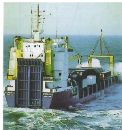
Stern door and ramp combined
