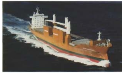
Multi-purpose ship "Schippersgracht" with its own cargo gear and loading ramps
