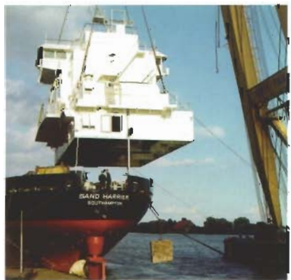
Installation of a complete deckhouse, while the ship is at the fitting out dock.
