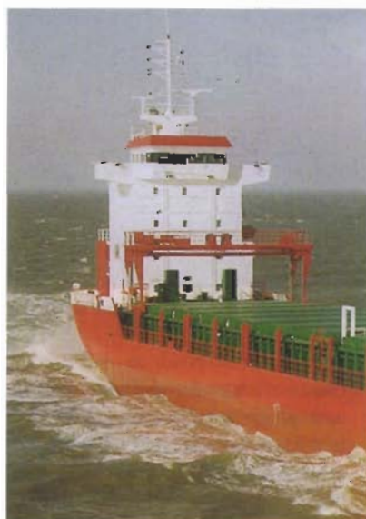
Multi-purpose ship with hatch cradle
