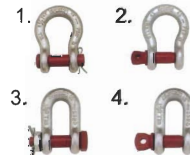
High tensile steel shackles. To obtain this high strength, after forging the shackles are subjected to heat treatment. (Quenched and Tempered)
