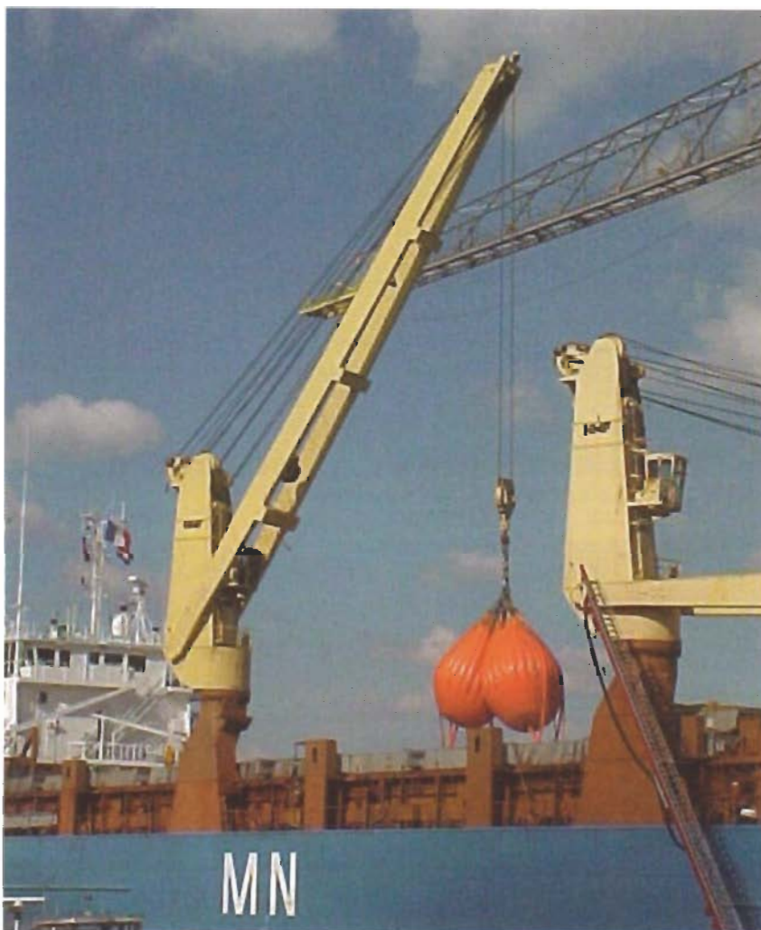
Testing the crane using water bags
