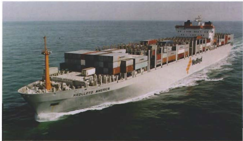
Nedlloyd America, an open cellular container ship L = 266 metres, B = 32 metres, 3,568 TEU
