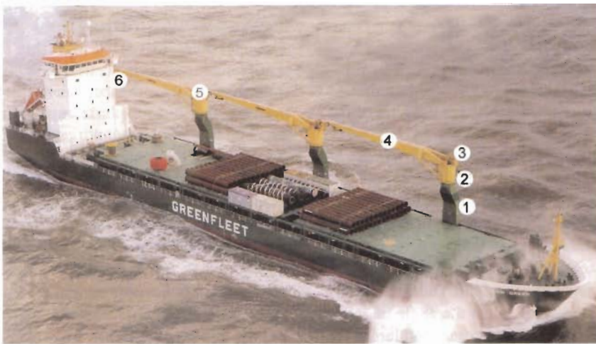
The crane jibs secured in their supports
