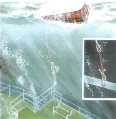
The sinking ship pulls the boat line and the raft is inflated.
