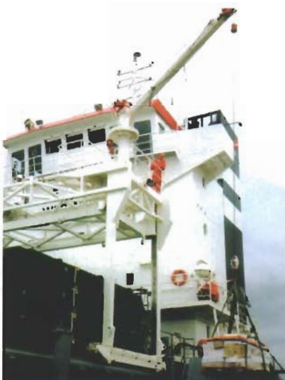
The storage crane lifting provisions on board
