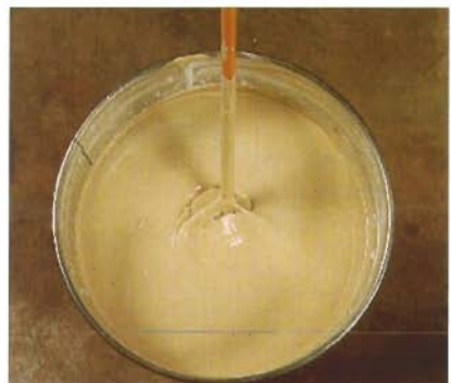
Mixing with a blender until the paint gets a uniform colour
