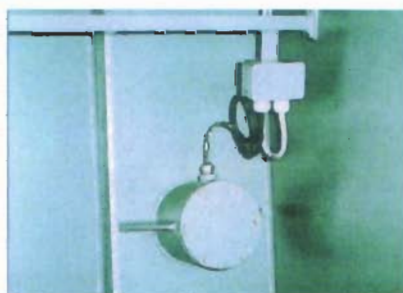
Reference electrode seen from inside
