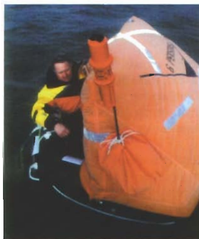
SART attached to the liferaft
