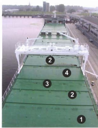
Multi-purpose ship with pontoon hatch covers
