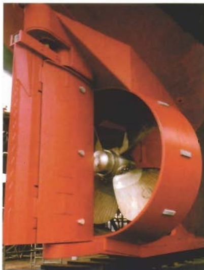
Setting in the heel of a flap rudder
