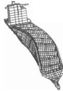
Waves coming in from starboard at an angle, torsion
