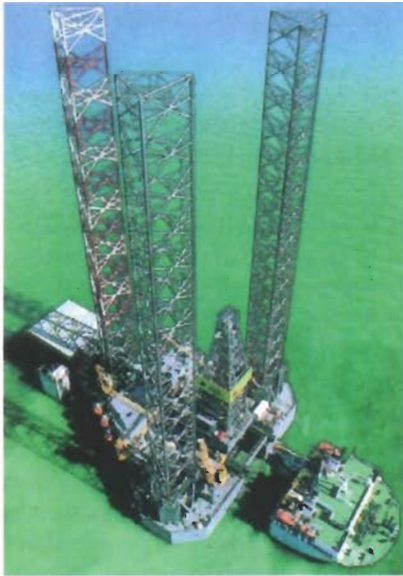
Semi-submersible ship loading a drilling rig.
