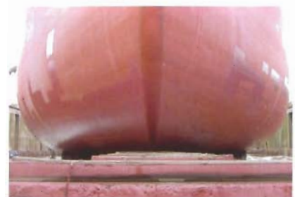
A ship with a large block-coefficient and a large midship section and prismatic coefficient.
