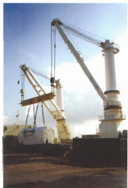
A medium-speed engine being loaded with own cargo gear
