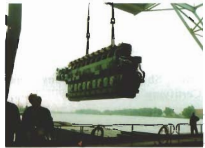
The main engine (70 tons ) is brought on board
