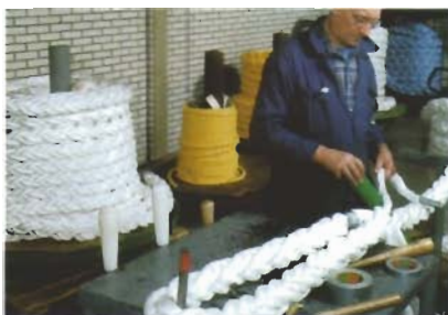
An eye is spliced into a rope
