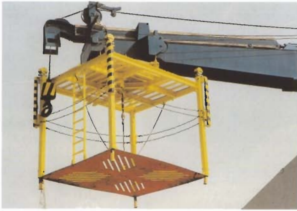
At the end of the pallet-swinger is a (yellow) pallet-cage
