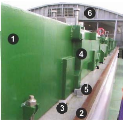
Pontoon hatch covers. Struts can be placed in the U-profiles to fasten the deckload
