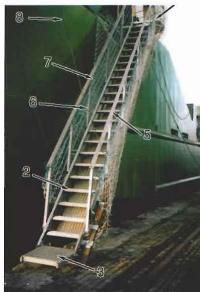
Unfolded accommodation ladder.
