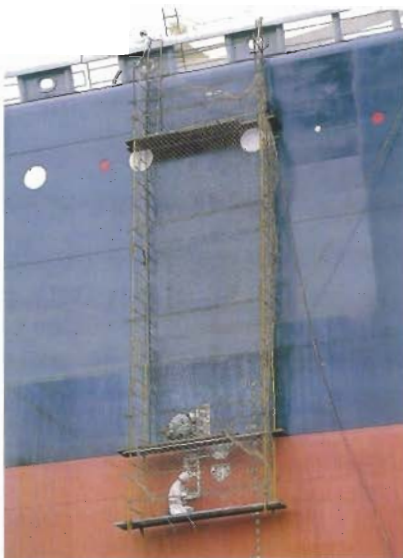
Survey to verify load lines on side of ship.
