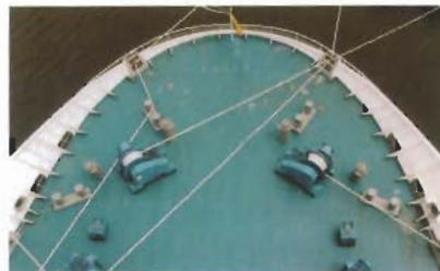
Winches on the forecastle and on the quarter deck of a car ferry
