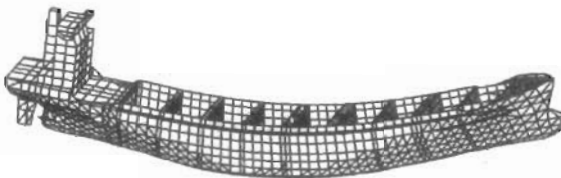
Ship on a wave top, hogging
