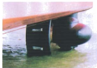
Sacrificial anodes on the propeller duct
