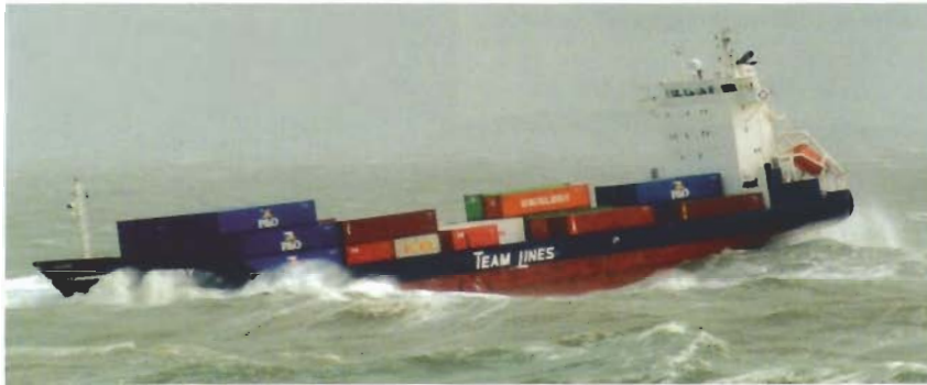
The ship is partially in a trough. In this case the foreship will experience a large sagging moment while the aft ship experiences a large hogging moment.
