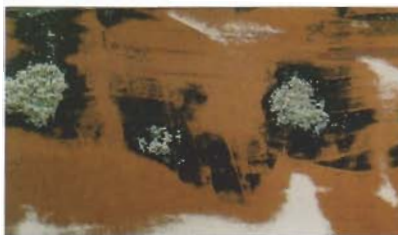
Fouling in places where the antifouling has gone
