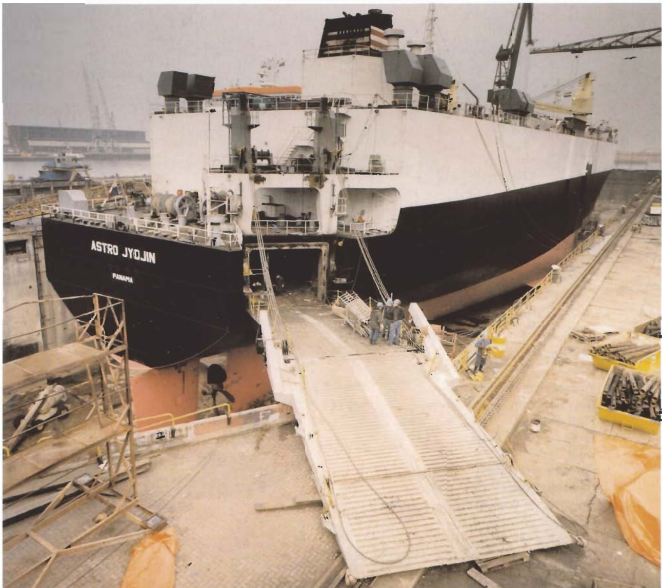
Ship with quarter ramp in dry-dock
