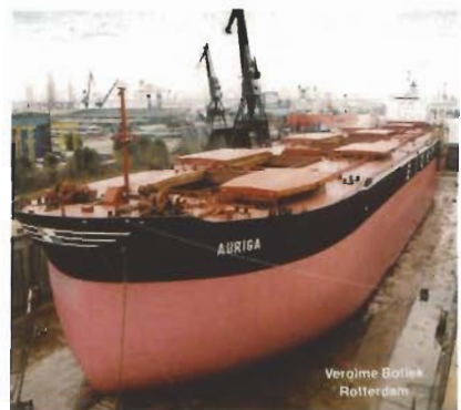
A ship with a small block-coefficient and a large midship section coefficient
