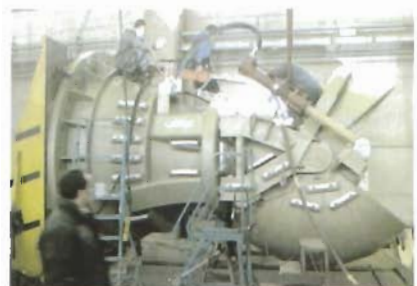
Waterjet with reversing bucket down
