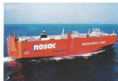
Ship with quarter ramp and straight ramp in the side
