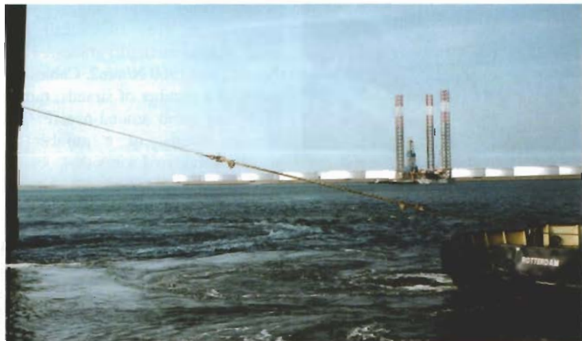
Towing wire with a stretcher
