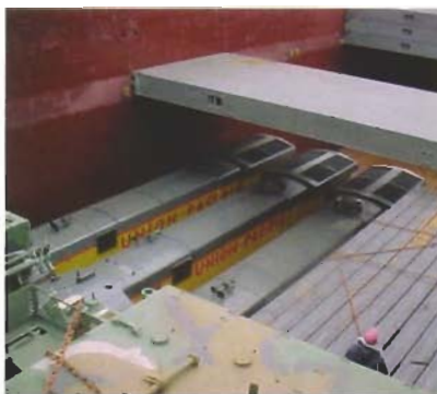
Pontoon hatches used as tween deck in a multi purpose ship
