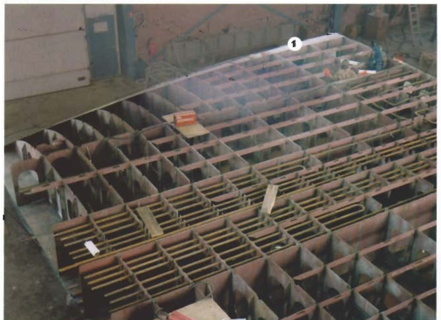
View of the down side of the double bottom. In the middle you can see the HFO-tank with heating coils.
