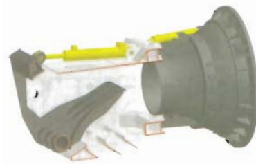
Side view of a water jet zero thrust
