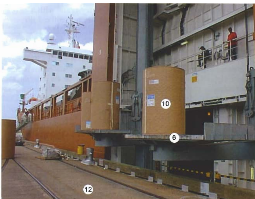
Paper rolls on the elevator. The cargo is transported by the lift to the tween deck or the lower hold
