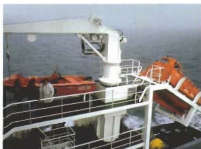
MOB -boat with crane. The crane can also bring the boat back on board.
