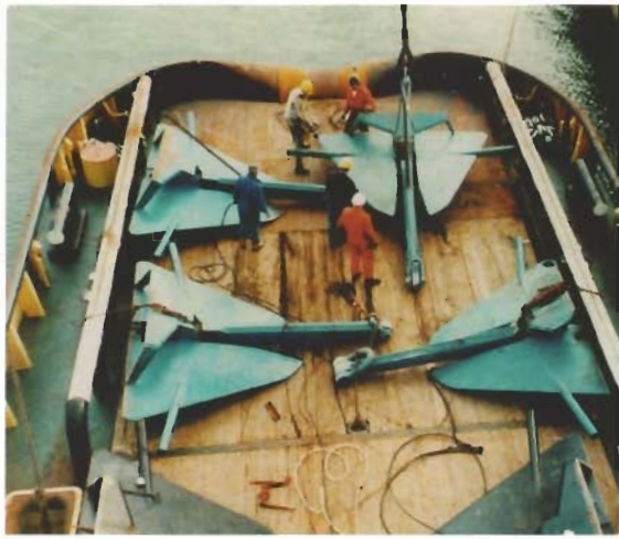
Flipper Delta-anchors on a deck of an AHTS
