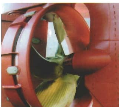
Fixed propeller in a wing-nozzle
