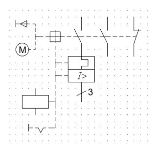
Three-pole mechanical switching device, operated by motor or manually, with trip-free mechanism, and: - thermal overload release
