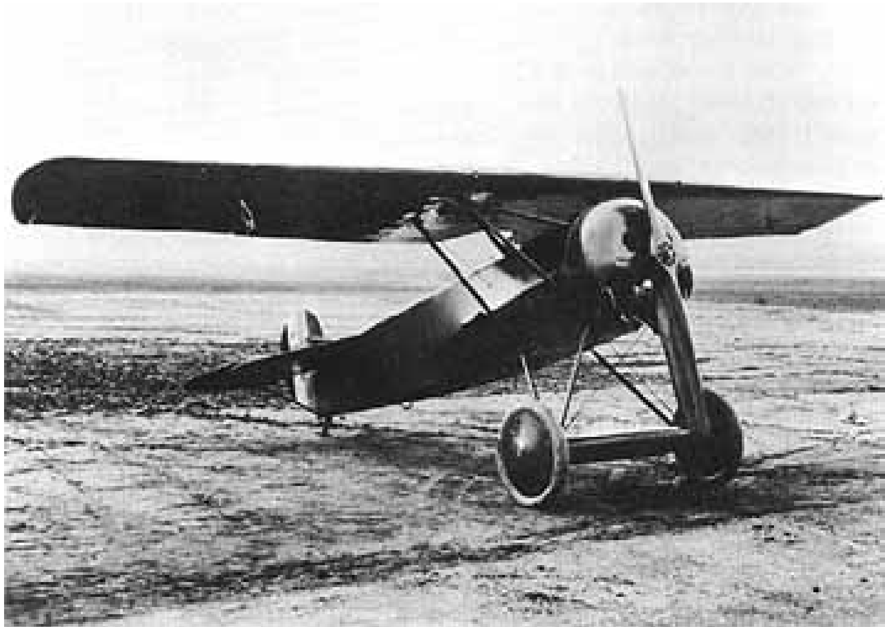
Fokker D-8, 1920 - torsional divergence
