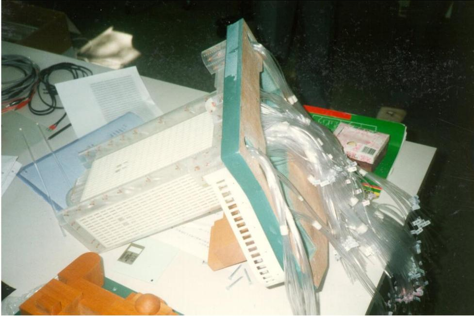
**Figure Q.3** – Pressure model with tubing.
