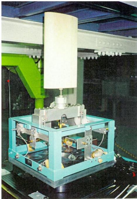
**Figure Q.9** –Building pivot model test.
