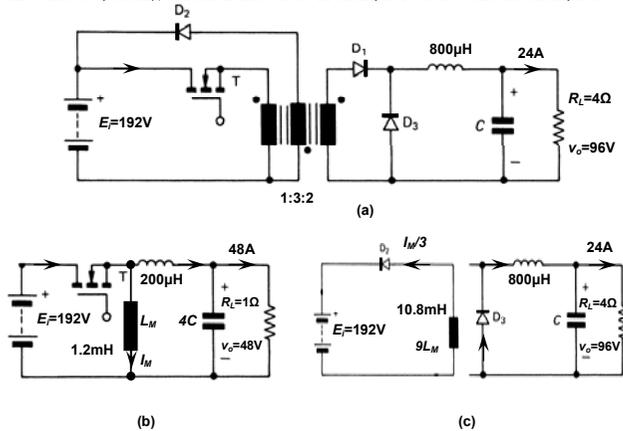
Figure 15.13. Isolated output forward converter and its equivalent circuits when the output is referred to the primary.
