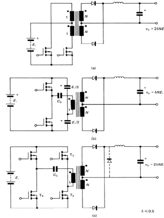
Figure 15.15. Multiple-switch, isolated output, pulse-width modulated converters: (a) push-pull; (b) half-bridge; and (c) full-bridge.
