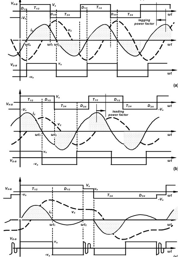
Figure 15.19. Three modes of series load resonant converter operation (a)  $f_s > f_o$ ; (b)  $1/2 f_o < f_s < f_o$ ; and (c)  $f_s < 1/2 f_o$ .
