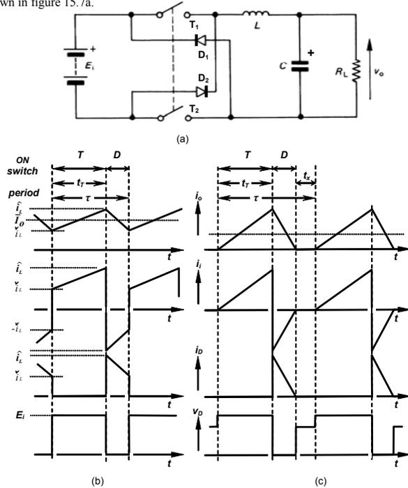
Figure 15.7. Basic reversible converter with  $\delta > 1/2$ :
