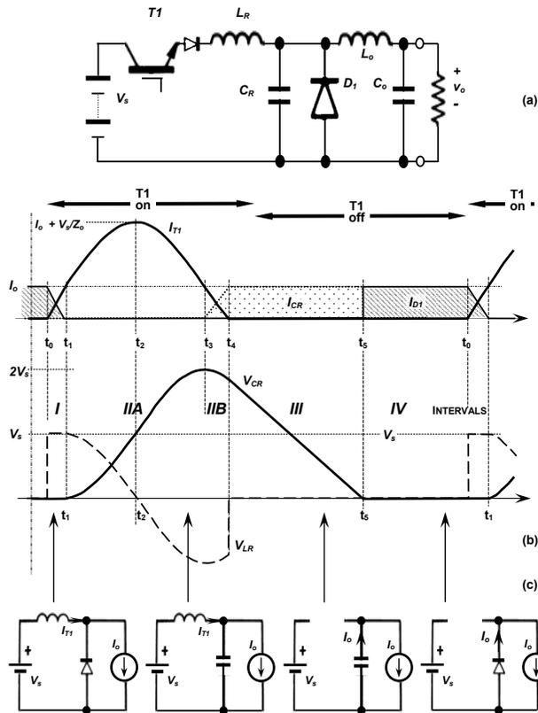
Figure 15.24. Zero current switching, ZCS, resonant switch dc to dc converter: (a) circuit; (b) waveforms; and (c) equivalent circuits.
