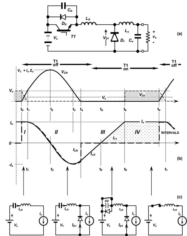
Figure 15.25. Zero voltage switching, ZVS, resonant switch dc to dc converter: (a) circuit; (b) waveforms; and (c) equivalents circuits.
