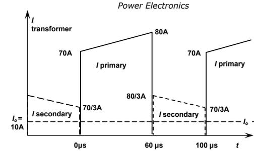
Figure 15.12. Currents for the transformer windings in example 15.7.
