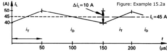
iv. The capacitor current is derived by using Kirchhoff's current law such that at any instant in time, the diode current, plus the capacitor current, plus the 30A constant load current into  $R$ , all sum to zero.
