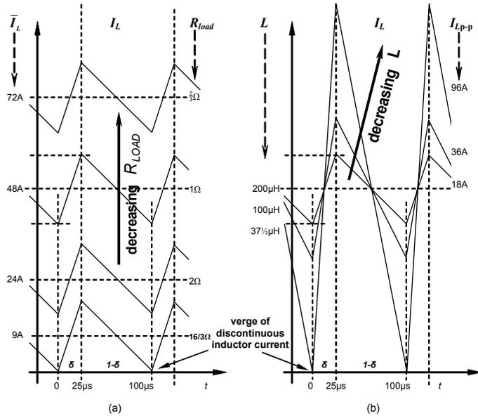
Figure 15.4. Forward converter (buck converter) operational mechanisms showing that: (a) the average inductor current is inversely proportional to load resistance  $R$  and (b) the inductor ripple current magnitude is inversely proportional to inductance  $L$ .
