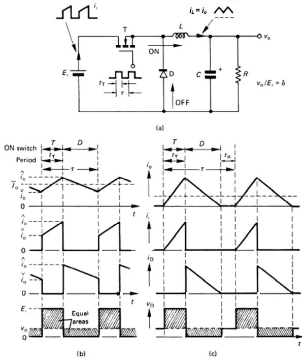
Figure 15.2. Non-isolated forward converter (buck converter) where  $v_o \leq E_i$ : (a) circuit diagram; (b) waveforms for continuous output current; and (c) waveforms for discontinuous output current.
