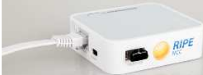
RIPE Atlas probe v3 TP-Link MR3020 router with custom firmware
