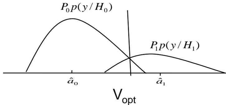
$$P_e = P_0 \int_{V_T}^{+\infty} p_y(y/H_0) dy + P_1 \left( 1 - \int_{V_T}^{+\infty} p_y(y/H_1) dy \right)$$
