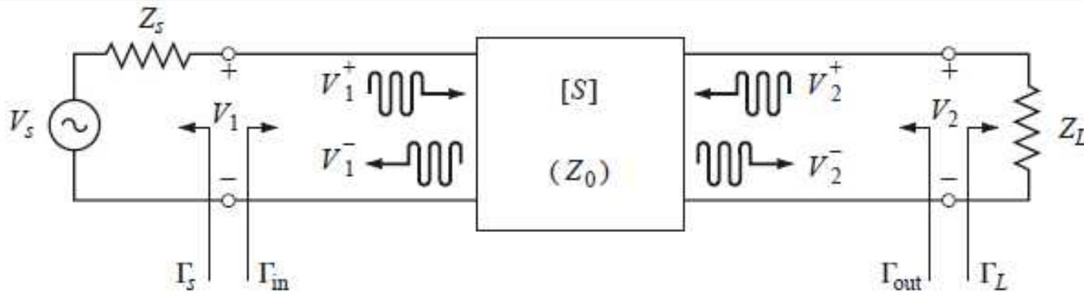
$$\Gamma_{in} = \frac{V_1^-}{V_1^+}$$
