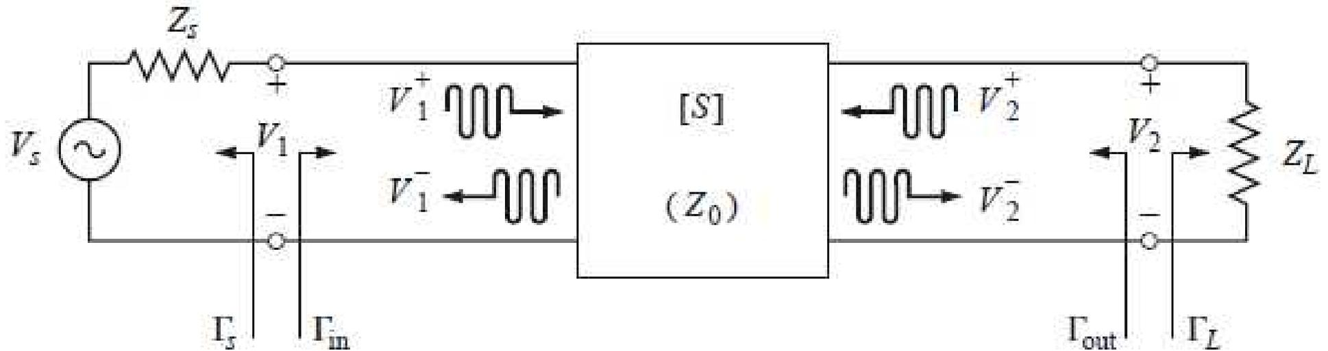
$$G_P = \frac{P_L}{P_{IN}} = \frac{\text{power delivered to the load}}{\text{power input to the network}}$$
