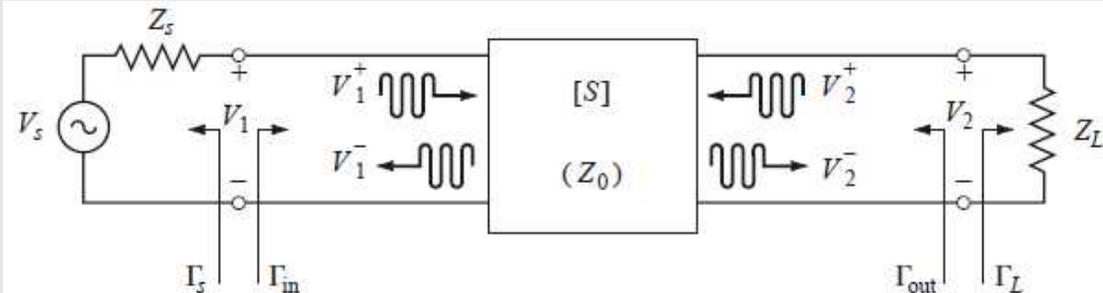
$$P_L = \frac{|V_S|^2 |S_{21}|^2 (1 - |\Gamma_L|^2) |1 - \Gamma_S|^2}{8Z_0 |1 - S_{22} \Gamma_L|^2 |1 - \Gamma_S \Gamma_{in}|^2}$$
