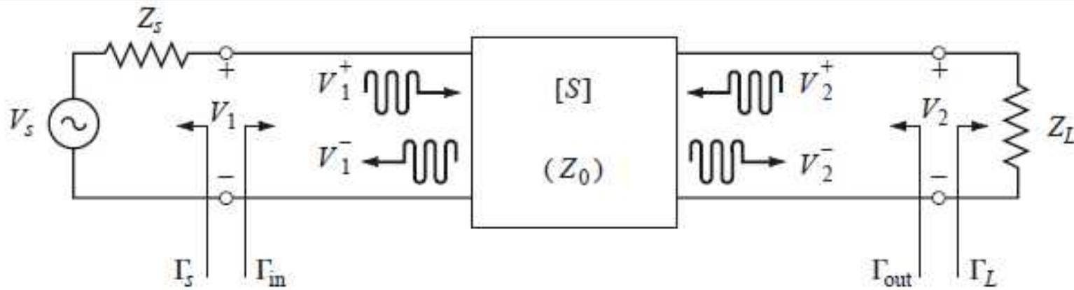
$$P^+ = \text{Re}\left[V_{rms}^+ \cdot I_{rms}^{+*}\right] = \frac{1}{2} \text{Re}\left[V^+ \cdot (I^+)^*\right] = \frac{1}{2} \text{Re}\left[V^+ \cdot \frac{(V^+)^*}{Z_0}\right] = \frac{1}{2} \frac{|V^+|^2}{Z_0} \quad \text{Potencia incidente}$$
