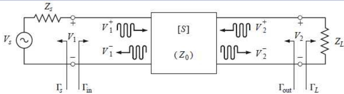
$$V_1 = V_S \frac{Z_{in}}{Z_S + Z_{in}} = V_1^+ + V_1^- = V_1^+ (1 + \Gamma_{in})$$
