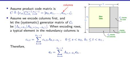
Redundancy columns are linear combinations of codewords in C<sub>2</sub> ⇒ they too are codewords in C<sub>2</sub>.
