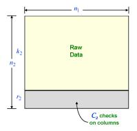
• Special case of a product code with  $k_1 = n_1$  (no redundancy on rows).
