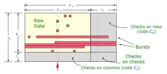
• Use part of the redundancy of  $C_h$  to attempt correction. In the figure, the marked column may be uncorrectble by  $C_v$  alone.
