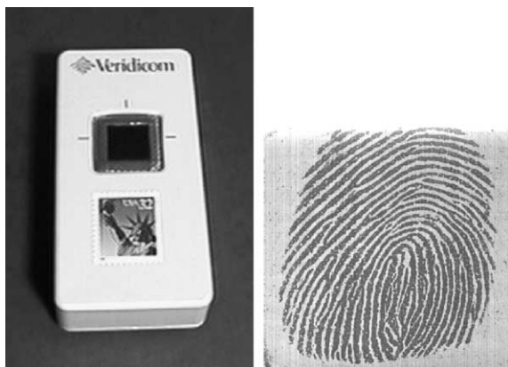
Fig. 4. A compact solid-state sensor and a sample fingerprint acquired by the sensor. The sensor is about the size of a postage stamp.
