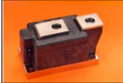
LS43_43 Single SCR POW-R-BLOK™ Module 430 Amperes / 1800-2200 Volts
