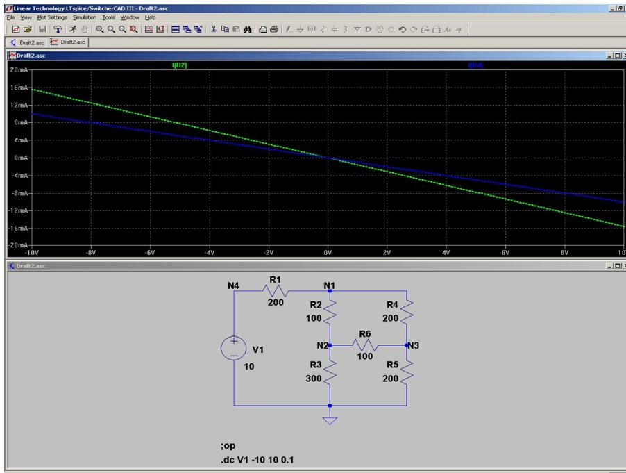
Figure 3.3 SWCAD screen with waveform viewer
