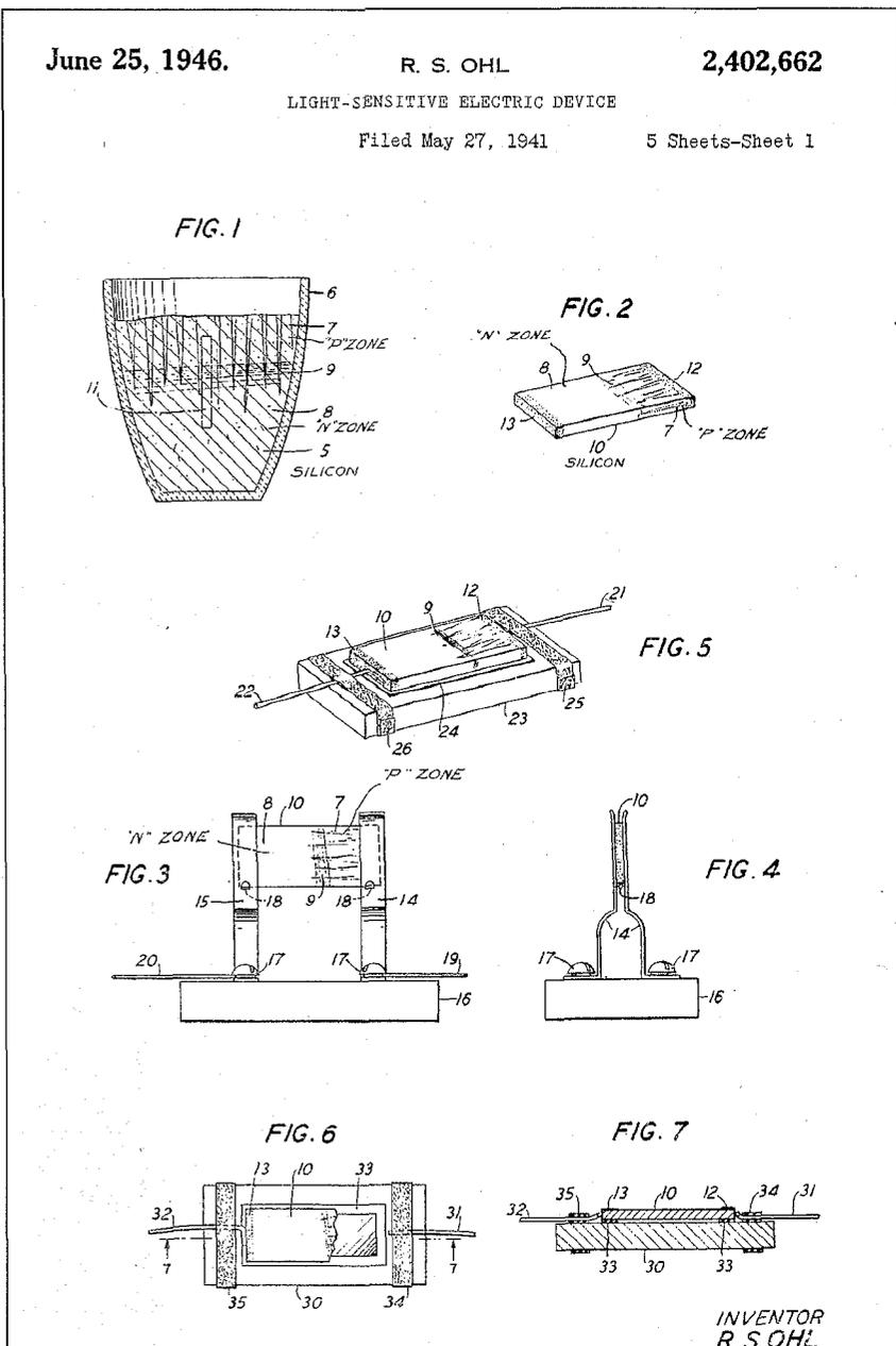
The patent application filed by Russell Ohl and Bell Telephone Laboratories for a "light-sensitive electric device" shows a cross section of an ingot of fused silicon [upper left] and an electromotive force cell made from the ingot [upper right]. Other drawings show ways of mounting the device.
