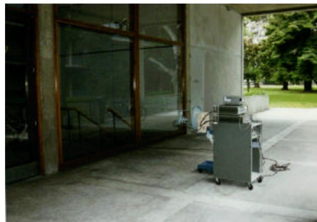
Measurement of propagation through building walls
