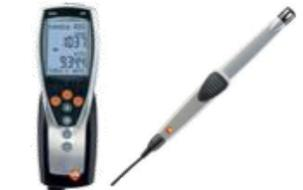
Non-dispersive infrared analyzer: CO<sub>2</sub>, T & RH
