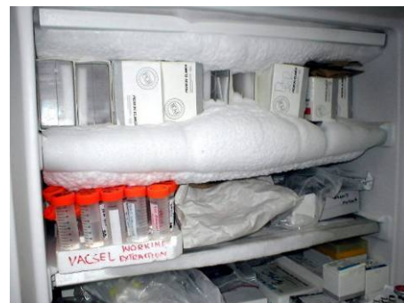
Photo 1.13 Ice piled up inside the freezer compartment
