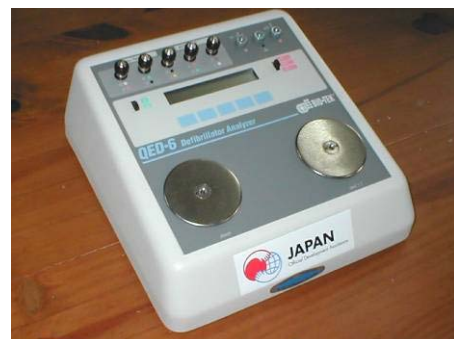
Photo 1.17 Example of a Defibrillator Analyser that is used to measure the power energy of defibrillators in periodic inspection
