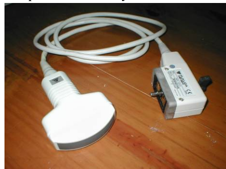
Photo 1.19 Example of a Convex type Ultrasonic Probe (electronic scanning), 3.5 MHz
