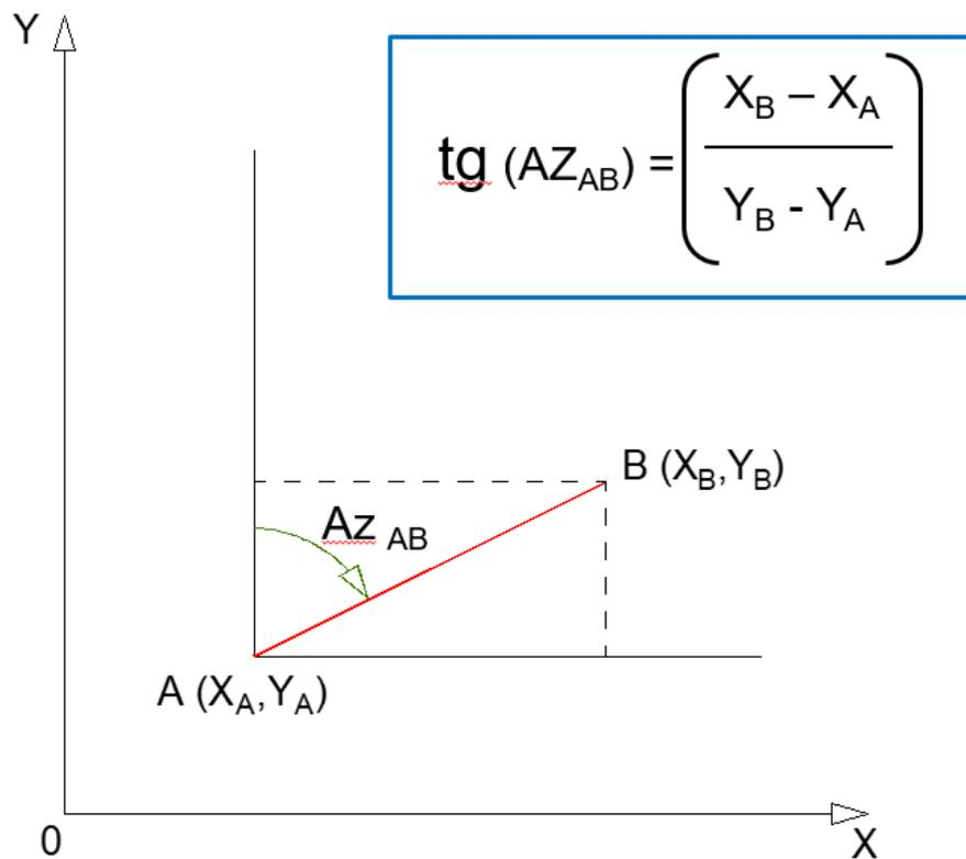
$$\Delta y > 0 \longrightarrow \underline{Az} = \underline{\text{Arctg}} \left( \frac{\Delta x}{\Delta y} \right) \left( + 360^\circ \text{ si } \underline{\Delta x} < 0 \right)$$
