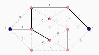
$$\phi(\mathbf{X}) = \left\{ \begin{array}{ll} 1 & \text{si } s \text{ y t est\'{a}n conectados} \\ 0 & \text{si } s \text{ y t no est\'{a}n conectados} \end{array} \right. \\ \rightarrow \left. \begin{array}{ll} \zeta &= \mathbb{P}\{\phi(\mathbf{X}) = 1\} \\ 1 - \zeta &= \mathbb{P}\{\phi(\mathbf{X}) = 0\} \end{array} \right.$$
