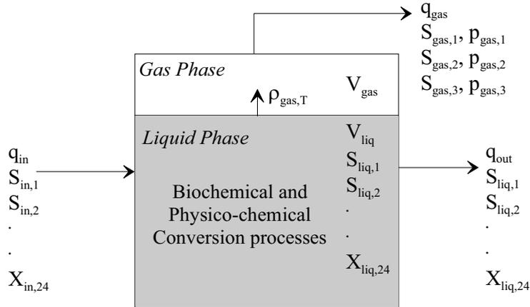
Figure 5.1: Schematic of a typical, single-tank digester.  $q$  = flow,  $\text{m}^3 \times \text{d}^{-1}$   $V$  = volume,  $\text{m}^3$ ;  $S_{\text{stream},i}$  = concentration of soluble components;  $X_{\text{stream},i}$  = concentration of particulate components (all in  $\text{kgCOD m}^{-3}$ );  $i$  is the component index (see Tables 3.1 and 3.2).
