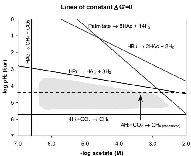
Figure 3.4: Lines of zero  $\Delta G'$  (298 K) for five reactions with similar assumptions to those in the caption to Figure 3.3 (except acetic acid concentration). The shaded portion shows regions where all reactions are possible. The measured hydrogen-utilising threshold and corresponding line (---) are based on Cord-Ruwisch *et al.* (1988).
