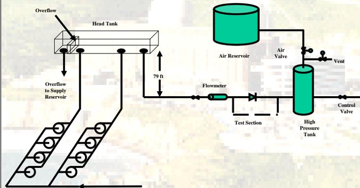
Example of one Large Bore Test Run
