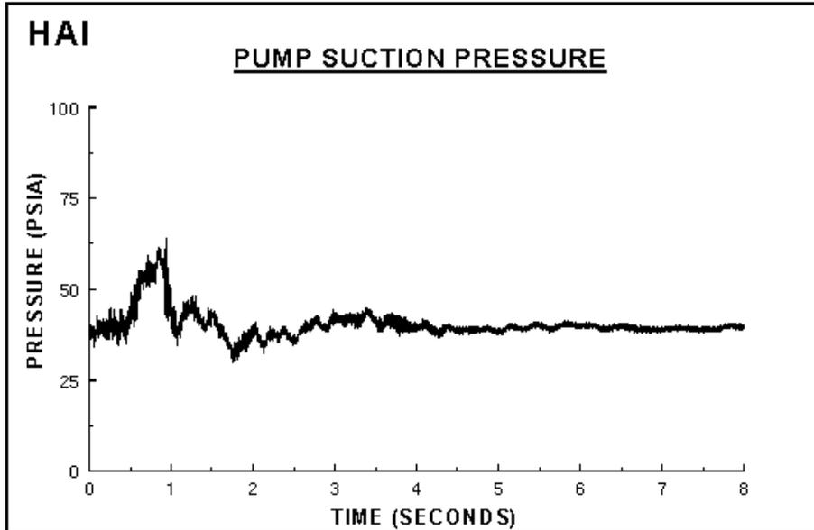
Figure (13) is a time expansion of the first 1.4 seconds of the data window. The most severe pressure oscillations occur at valve closure (0.9200 seconds).
