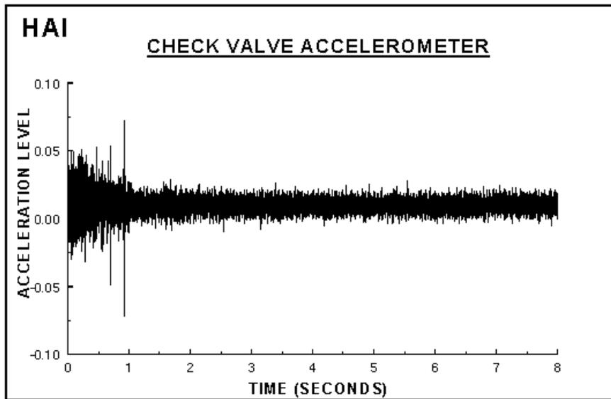
Figure (15) is the time expansion of the accelerometer trace for the first 1.5 seconds of the data window and shows the valve closure at 0.9200 seconds.
