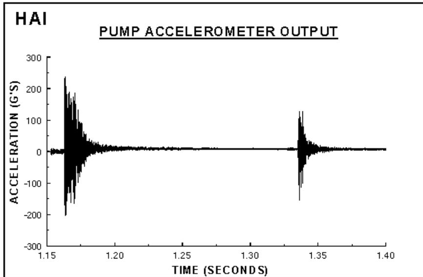
Figure (7) shows an expansion of the time around the first shock. Note the increase in vibration at 1.1530 seconds prior to the major shock at 1.1630 seconds. If this is interpreted as motion of the valve it indicates an extremely short period of valve motion (0.010 seconds).
