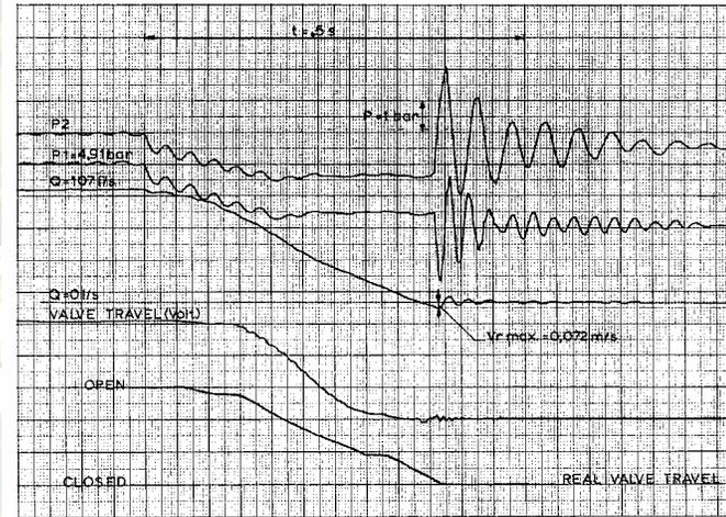
Axial Flow Check Valve Dynamic Testing
