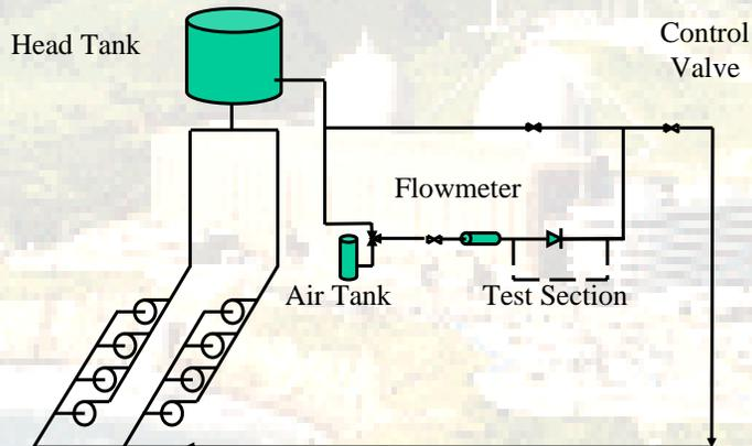
Axial Flow Check Valve Dynamic Testing
