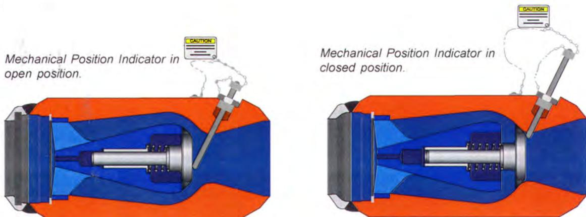
*Normally Closed NOZZLECHECK Valves with Position Indicator for operational verification in-place. Meets 89-04 IST requirements (reduced outage time by requiring the removal of only one pipe plug.).*
