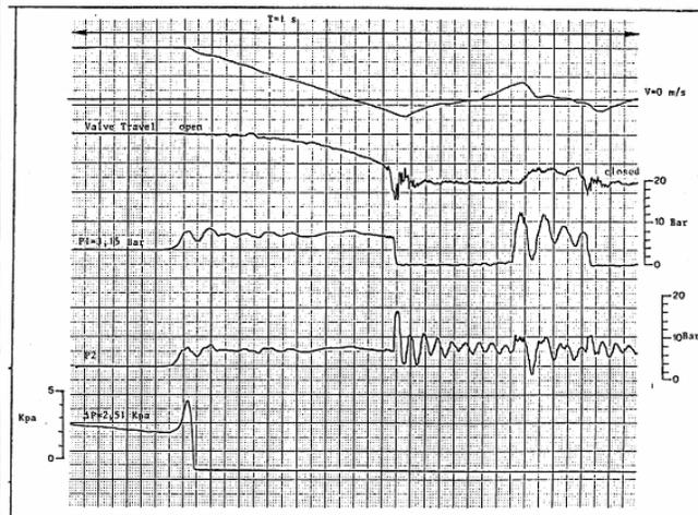
Small Bore Test Loop-Upstream Venting
