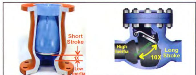
Short Stroke: NOZZLECHECK vs Swing Check
