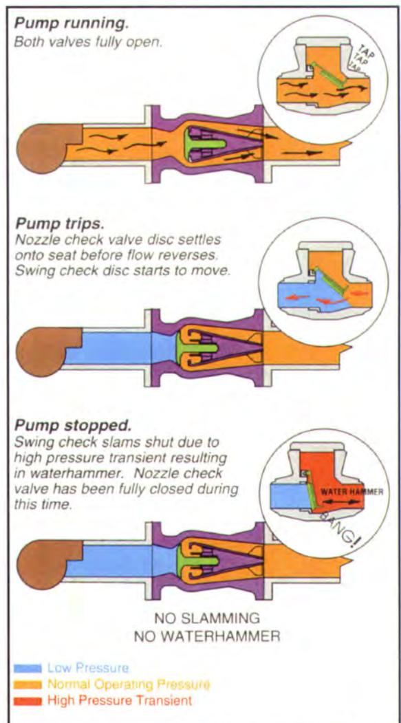
Operational Comparison of NOZZLECHECK and Swing Check Valves.
