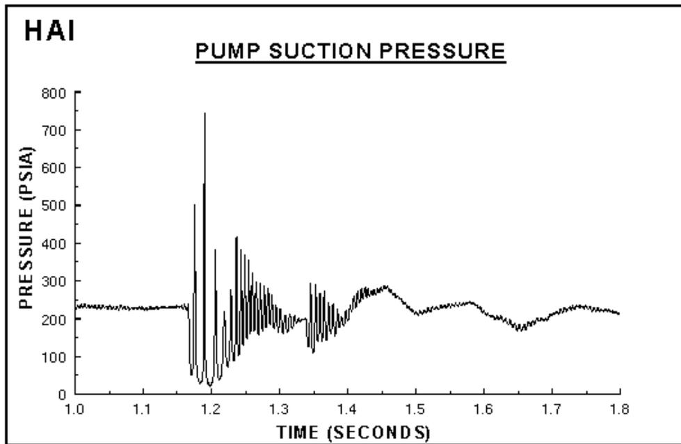
The remainder of the data set showed large pipe motion and high structural loading of the support system. As a result, the decision was made to install in-line nozzle check valves to reduce transient loading on the piping system.
