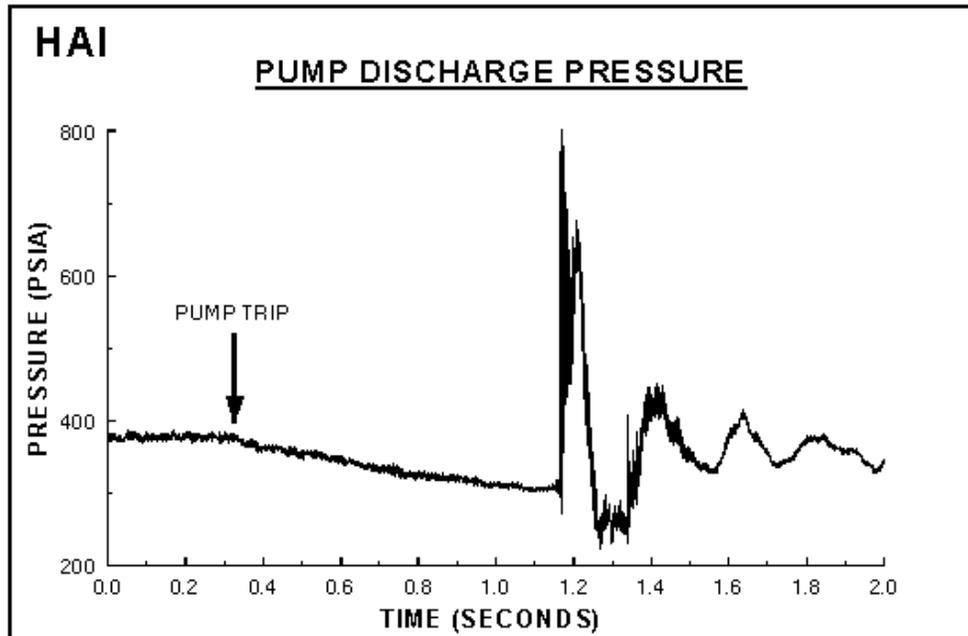
Figure (5) expands the time scale after the first reaction at 1.1650 seconds with a second reaction at 1.3380 seconds. The initial reaction shows high frequency high amplitude waves consistent with water hammer phenomena resulting from a rapid blockage of reverse flow by the check valve
