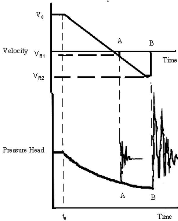
Velocity and Pressure History after a pump trip, downstream of the discharge check valve. The "A" check valve closes faster, with a lower  $V_{R1}$ , and much smaller pressure rise. The "B" check valve closes slower, with a higher  $V_{R2}$ , resulting in a higher pressure rise.
