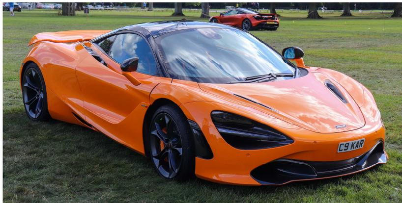
According to McLaren the 720S can accelerate to 100 km/h (62 mph) in 2.9 seconds, to 200 km/h (124 mph) in 7.8 seconds, can achieve a maximum speed of 341 km/h (212 mph), and has a 0.25 mile (402 m) time of 10.3 seconds. It has 710 horsepower.
