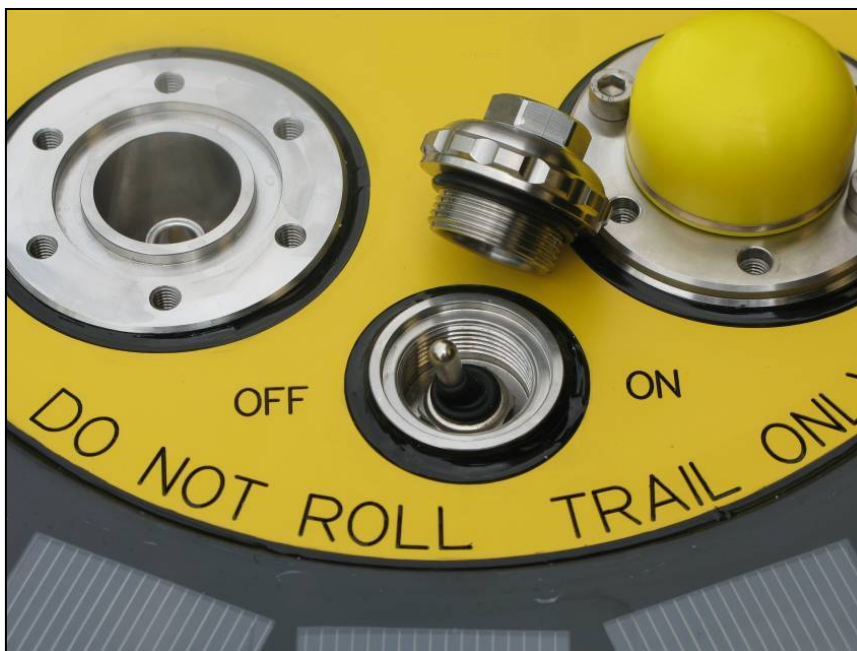
Figure 5.10.2. External power switch on the hatchcover
