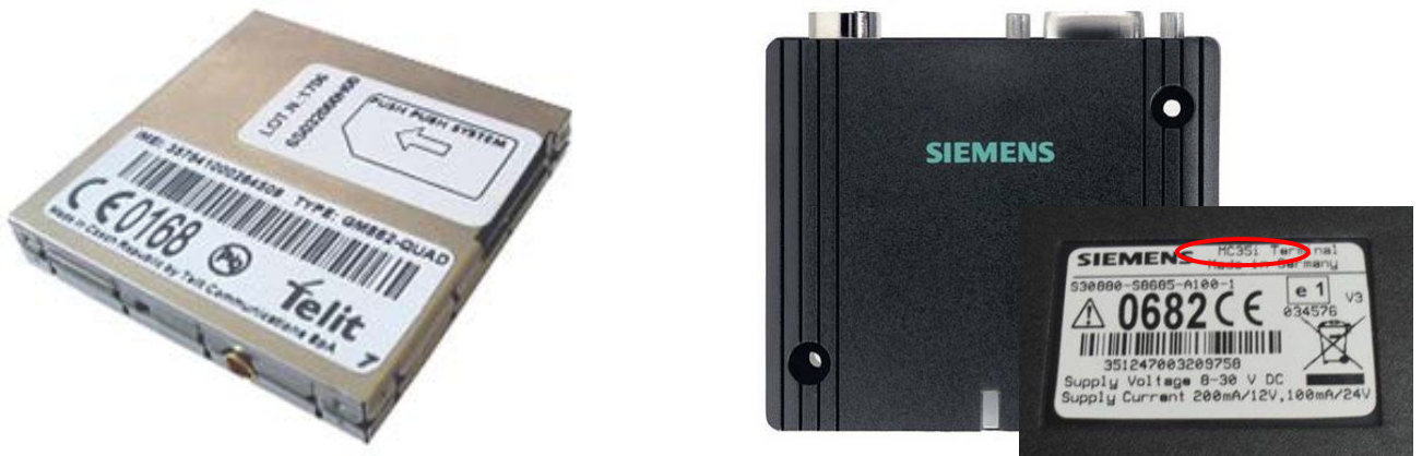
Fig 5.17.4 Photographs of Telit and Siemens GSM modems used in Waverider buoys. As for the Siemens modem the particular model is critical. Check the label on the bottom side (area inside red ellipse).
