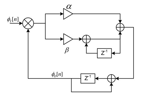
In the figure of the control loop above, we want to find the transfer function, so we solve for:
