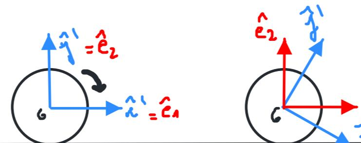
$$\begin{aligned} \{i, j, k\} & \quad \{x_1, x_2, x_3\} \\ I_e &= I_e = \frac{M R^2}{4} \begin{pmatrix} 1 & 0 & 0 \\ 0 & 1 & 0 \\ 0 & 0 & 2 \end{pmatrix} \end{aligned}$$
