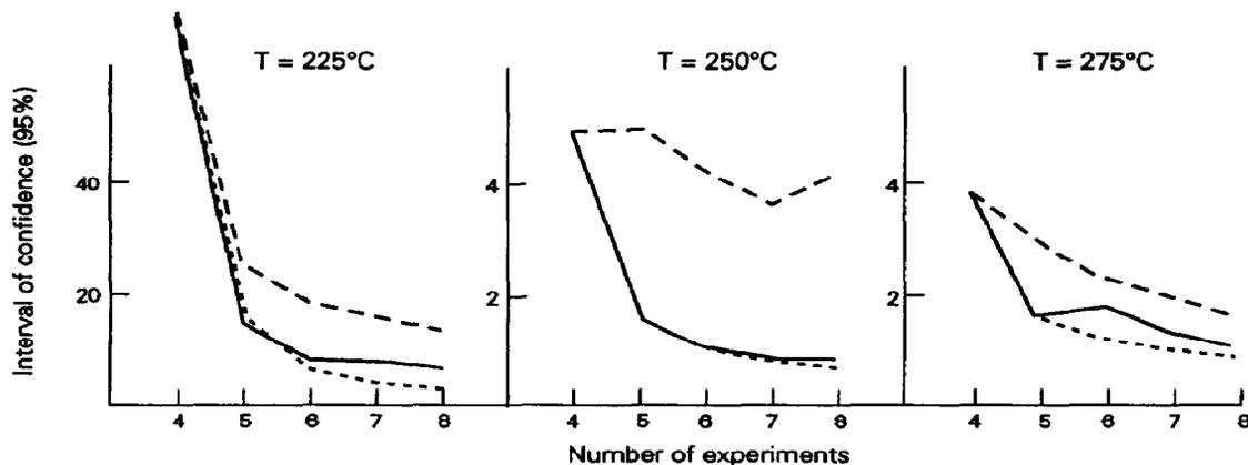
Fig. 3. Evolution of confidence limits of  $k_R$ . (—)  $y$ -trace design and volume design, (---) simple volume design, (.....)  $\beta$ -trace design and shape design.
