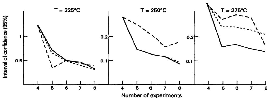
Fig. 2. Evolution of confidence limits of  $k_A$ . (—)  $y$ -trace design and volume design, (---) simple volume design, (.....)  $\beta$ -trace design and shape design.
