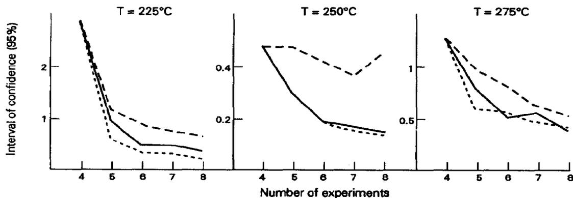
Fig. 1. Evolution of confidence limits of  $k$ . (—)  $y$ -trace design and volume design, (---) simple volume design, (.....)  $\beta$ -trace design and shape design.
