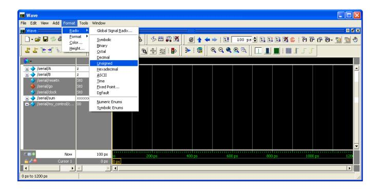
Figure 20. Changing the radix of A, B and sum signals.
