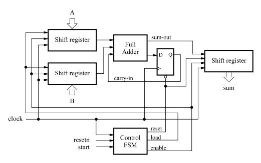
Figure 2. Block diagram of a serial-adder circuit.
