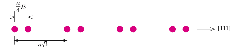
Fig. 2.5. Arrangement of atoms along the [111] direction of the diamond crystal. Notice that the crystal is invariant under inversion either with respect to the midpoint between the atoms or with respect to one of the atoms followed by an appropriate translation along the [111] axis
