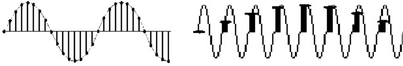
Figure 2.5 The relationship between the least sampling interval and the highest functional frequency. Left: sampling interval is less than half the functional frequency so that full reconstruction is possible; right: sampling interval is larger than half the functional frequency so that information about the function is lost.
