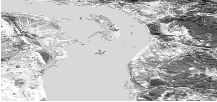
Figure 12.17 Mapping texture onto the surface of DTM. The color plate can be viewed at http://www.crcpress.com/e_products/downloads/download.asp?cat_no=TF1732 .
