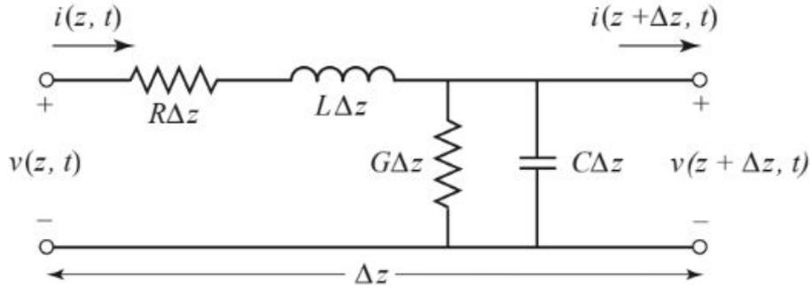
$$\frac{\partial v(z, t)}{\partial z} = -Ri(z, t) - L \frac{\partial i(z, t)}{\partial t},$$
