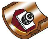
Circumferential Inside Diameter
