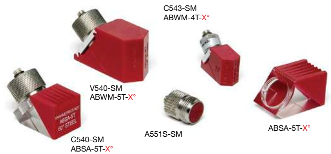
Miniature angle beam transducers and wedges are used primarily for testing weld integrity. Their design enables them to be easily scanned back and forth and provides a short approach distance.
