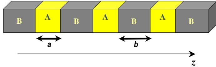
$$-\frac{\alpha^2 + \beta^2}{2\alpha\beta} \text{sen}(\alpha a) \text{sen}(\beta b) + \text{cos}(\alpha a) \text{cos}(\beta b) = \text{cos}(k(a + b)) \quad (11)^9$$
