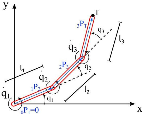
$$\text{ART 1: } \omega_1 = \dot{\theta}_1 \cdot z_1 \mid v_1 = \dot{d}_1 \cdot z_1$$
