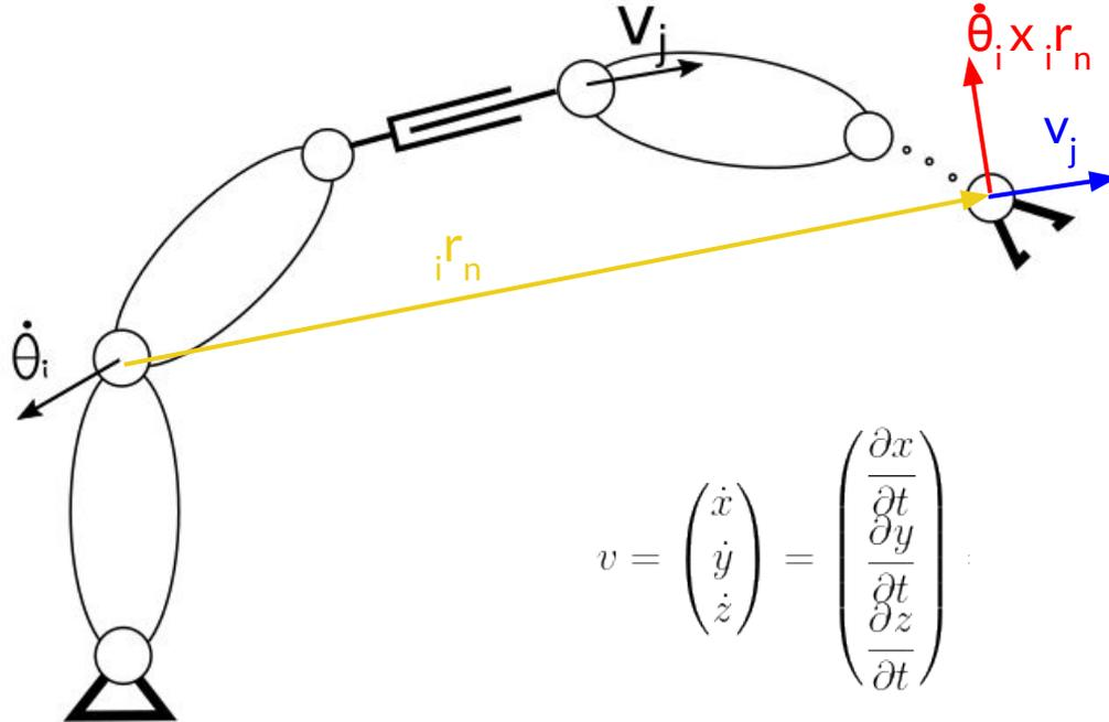
$$v = \begin{pmatrix} \dot{x} \\ \dot{y} \\ \dot{z} \end{pmatrix} = \begin{pmatrix} \frac{\partial x}{\partial t} \\ \frac{\partial y}{\partial t} \\ \frac{\partial z}{\partial t} \end{pmatrix} :$$
