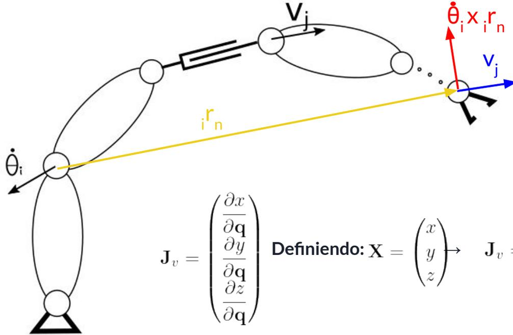
$$J_v = \begin{pmatrix} \frac{\partial x}{\partial q} \\ \frac{\partial y}{\partial q} \\ \frac{\partial z}{\partial q} \end{pmatrix}$$
