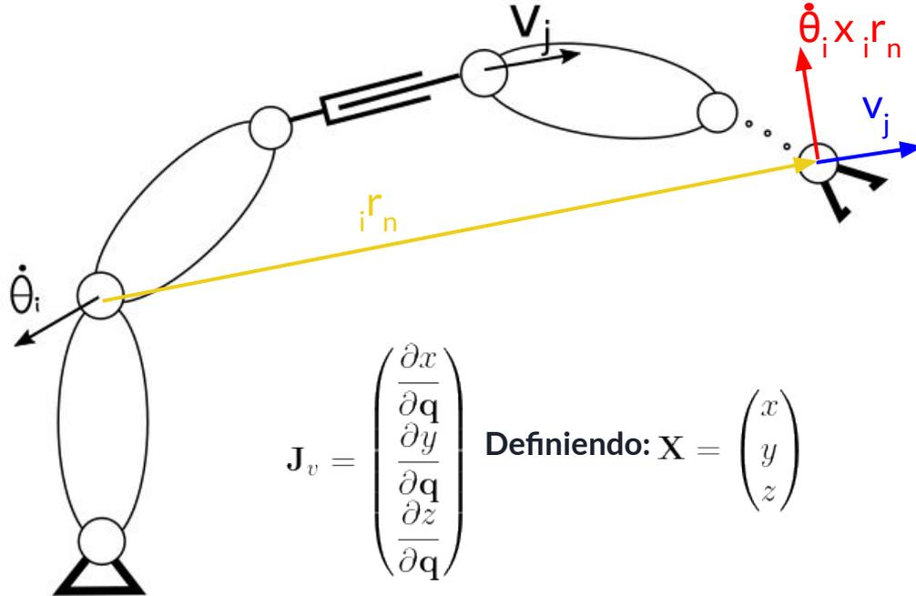
$$J_v = \begin{pmatrix} \frac{\partial x}{\partial \mathbf{q}} \\ \frac{\partial y}{\partial \mathbf{q}} \\ \frac{\partial z}{\partial \mathbf{q}} \end{pmatrix} \quad \text{Definiendo: } \mathbf{X} = \begin{pmatrix} x \\ y \\ z \end{pmatrix}$$
