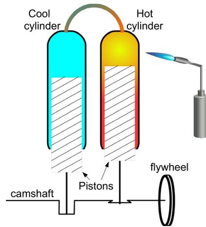
Fig. 2. Simple model of the Stirling engine; it uses two disposable glass syringes as a piston-cylinder system (see Ref. 10).
