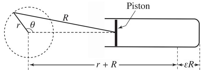
Fig. 3. Constraint scheme between the volume of gas in the cylinder and the camshaft angle  $\theta$ . The circle represents the cam rotation. The piston is considered to have a negligible thickness.
