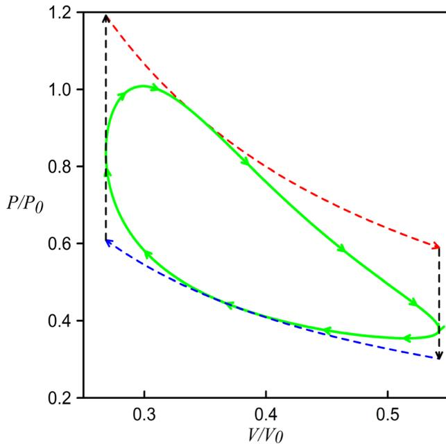
Fig. 1. Dimensionless pressure-volume diagram. The alternative Stirling cycle is presented as the solid curve (green online) compared to the usual Stirling cycle shown as the dashed cycle. The arrows indicate the evolution with increasing  $\theta$ . The parameters values are  $\phi = 5.2\pi$ ,  $\alpha = 10$ ,  $\beta = 1.33$ ,  $\varepsilon = 0.1$ , and  $z = 0.1$ .
