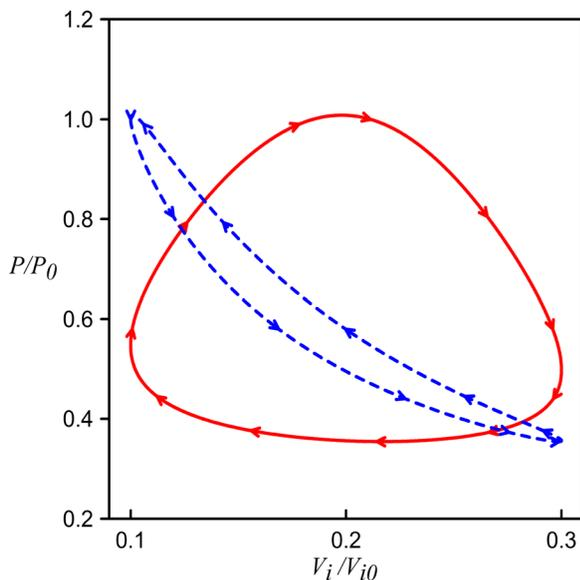
Fig. 4. Dimensionless pressure-volume diagram for the hot gas (solid curve, red online) and the cool gas (dashed curve, blue online). For the hot (cool) gas, the abscissa axis is  $V_2/V_{20}$  ( $V_1/V_{10}$ ). The arrows indicate the evolution with increasing  $\theta$ . The values of the parameters are the same as in Fig. 1.
