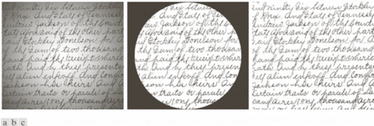
FIGURE 10.49 (a) Text image corrupted by spot shading. (b) Result of global thresholding using Otsu's method. (c) Result of local thresholding using moving averages.
