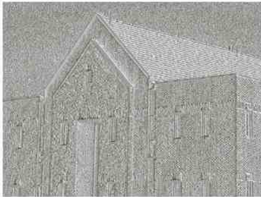
FIGURE 10.17 Gradient angle image computed using Eq. (10.2-11). Areas of constant intensity in this image indicate that the direction of the gradient vector is the same at all the pixel locations in those regions.
