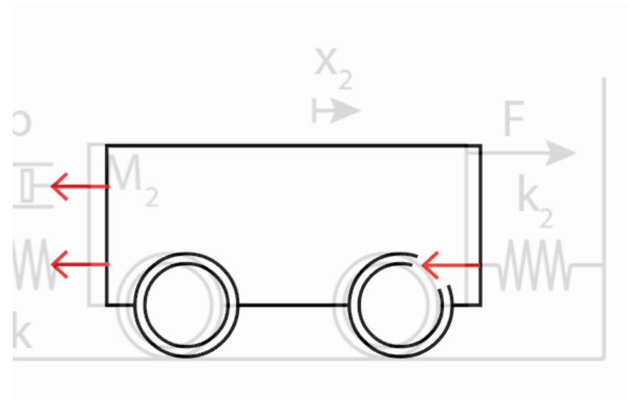
$$2^{\text{a}} \text{ Ley de Newton) } M_2 \ddot{x}_2 = k \left( (x_1 - x_2) - (l_0^1 - l_0^2) \right) + b(\dot{x}_1 - \dot{x}_2) - k_2(x_2 - l_0^2) + F_{ext}$$
