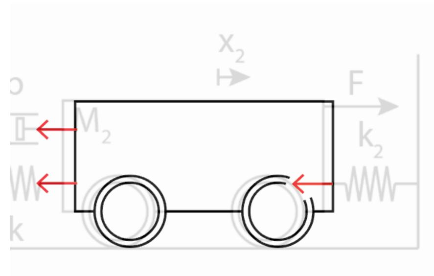
$$2^a \text{ Ley de Newton) } M_2 \ddot{x}_2 = k \left( (x_1 - x_2) - (l_0^1 - l_0^2) \right) + b(\dot{x}_1 - \dot{x}_2) - k_2(x_2 - l_0^2)$$
