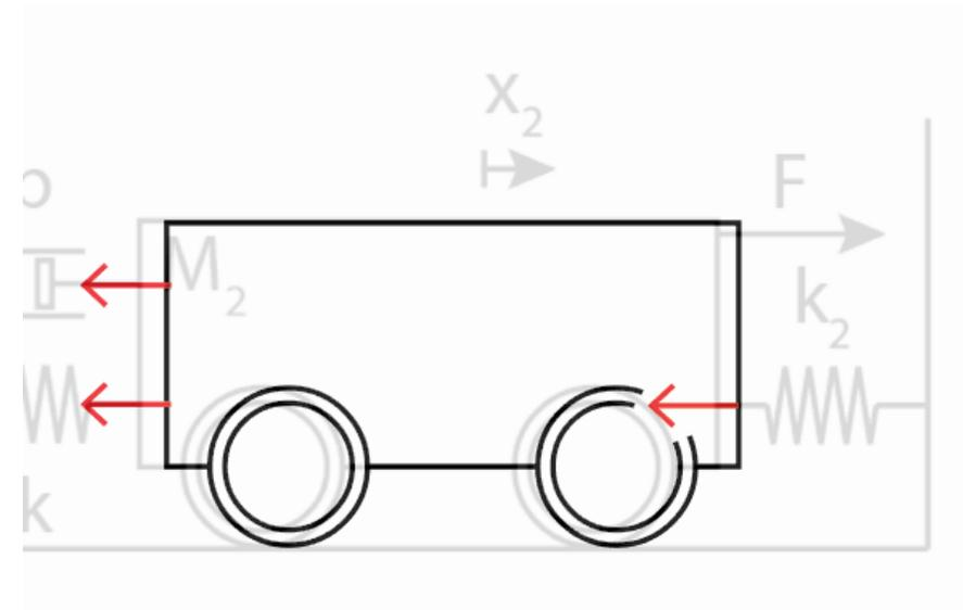
$$2^{\text{a}} \text{ Ley de Newton) } M_2 \ddot{x}_2 = k \left( (x_1 - x_2) - (l_0^1 - l_0^2) \right) + b(\dot{x}_1 - \dot{x}_2)$$
