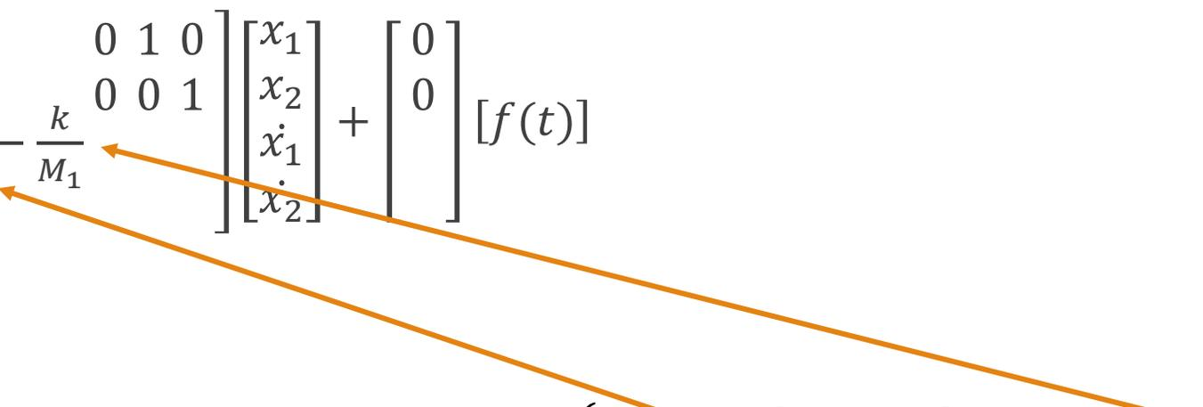
$$\begin{cases} \ddot{x}_1 = -\frac{k_1}{M_1} x_1 - \frac{b}{M_1} (\dot{x}_1 - \dot{x}_2) - \frac{k}{M_1} (x_1 - x_2) \\ \ddot{x}_2 = \frac{k}{M_2} (x_1 - x_2) + \frac{b}{M_2} (\dot{x}_1 - \dot{x}_2) - \frac{k_2}{M_2} x_2 + \frac{F_{\text{ext}}}{M_2} \end{cases}$$
