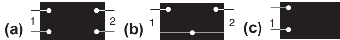
Figure 8.1: Black boxes. The two boxes (a) and (b) allow for transfer parameters from one port to the other. Box (c) is a one-port, two-terminal box with only driving point parameters possible.
