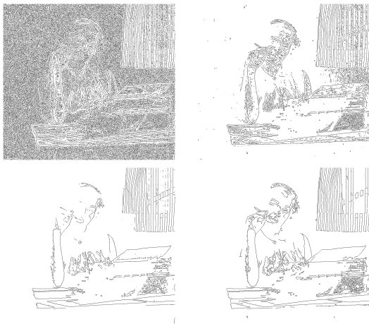
Figure: Different threshold values for the Non Maximal Suppression step of the Canny filter: 0.1, 2, 10 and 2 threshold with hysteresis with values 2 and 10
