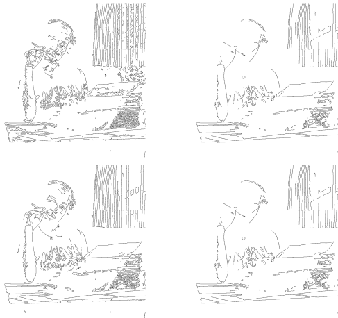
Figure: Canny edge detector with different thresholds in the hysteresis step of the algorithm. (a) Th_{low} = 1 and Th_{high} = 5 , (b) Th_{low} = 1 and Th_{high} = 20 , (c) Th_{low}=2 and Th_{high} = 10 , (d) Th_{low}=2 and Th_{high}=20 . Note how all the set of parameters give some non meaningful contours.
