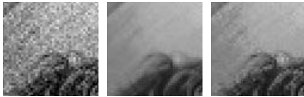
FIG. 12. Optimal correction experience. Left: Noisy image. Middle: NL-means solution. Right: NL-means corrected solution. The average with the noisy image makes the solution noisier, but details and fine structure are better preserved.
