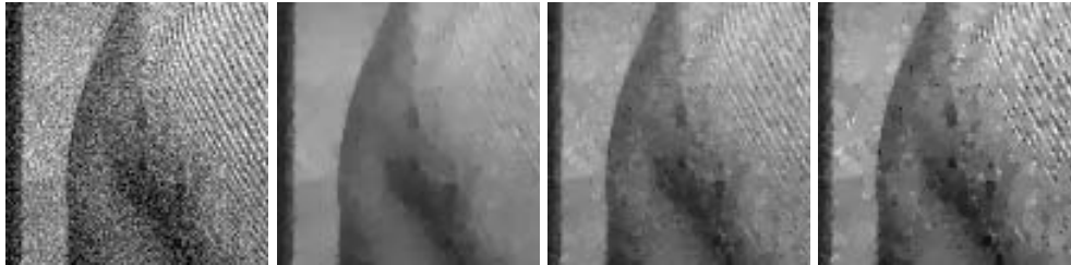
FIG. 22. Denoising experience on a natural image. From left to right and from top to bottom: noisy image (standard deviation 25), the total variation minimization, the Tadmor-Nezzar-Vese iterated total variation, and the Osher et al. iterated total variation.
