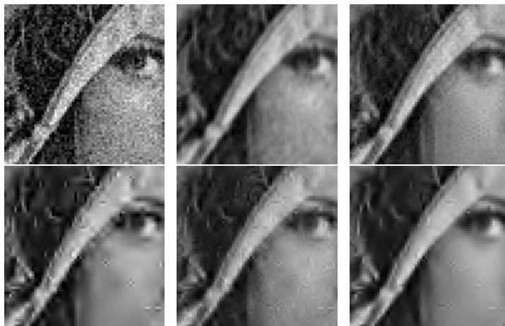
FIG. 5. Denoising experiment on a natural image. From left to right and from top to bottom: noisy image (standard deviation 20), Fourier–Wiener filter (ideal filter), the DCT empirical Wiener filter, the wavelet hard thresholding, the soft wavelet thresholding, and the translation invariant wavelet hard thresholding.
