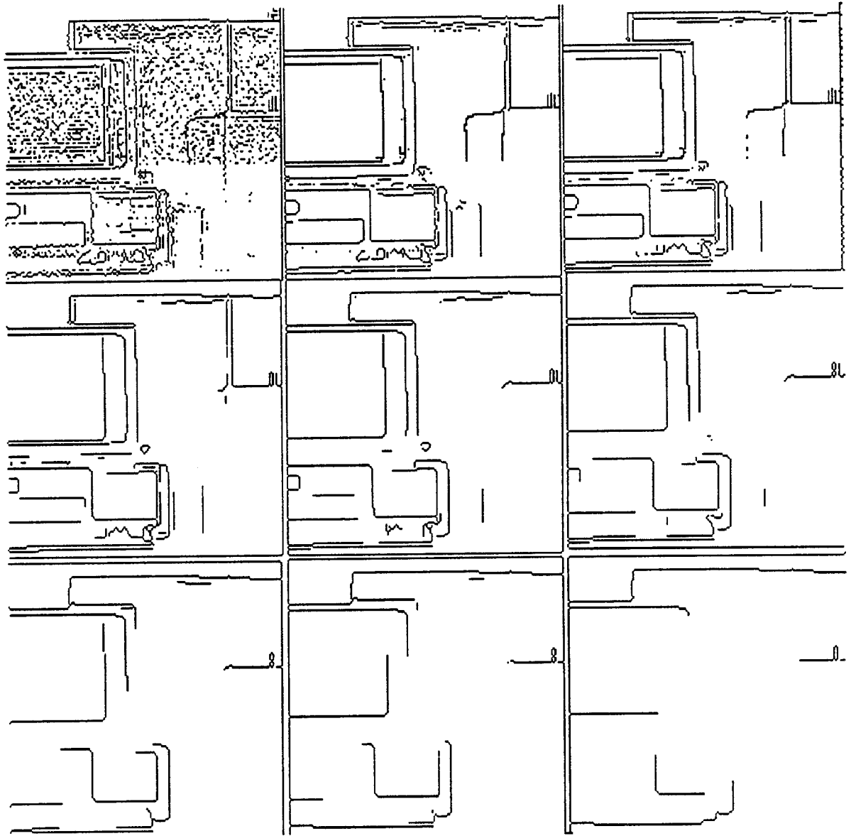
Figure 16: Edges detected on figure 13 using a thinning and linking stage [4].
