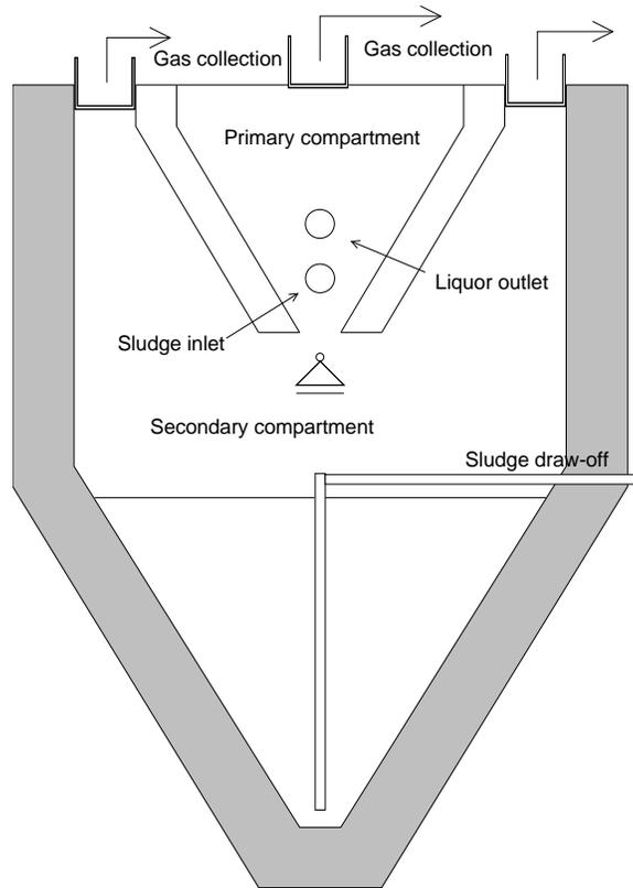
**Figure 26. Experimental two-stage garbage digester**
