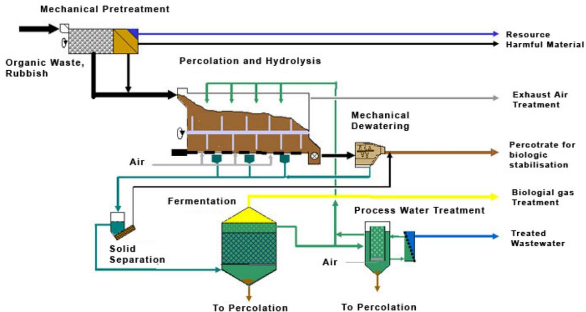
**Figure 20. Schematic waste-flow diagram of the two-stage Biopercolat process**
