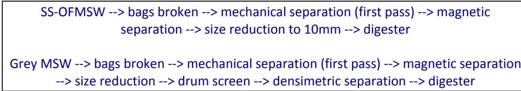
**Figure 7. Bassano, Italy pre-processing diagram.**
