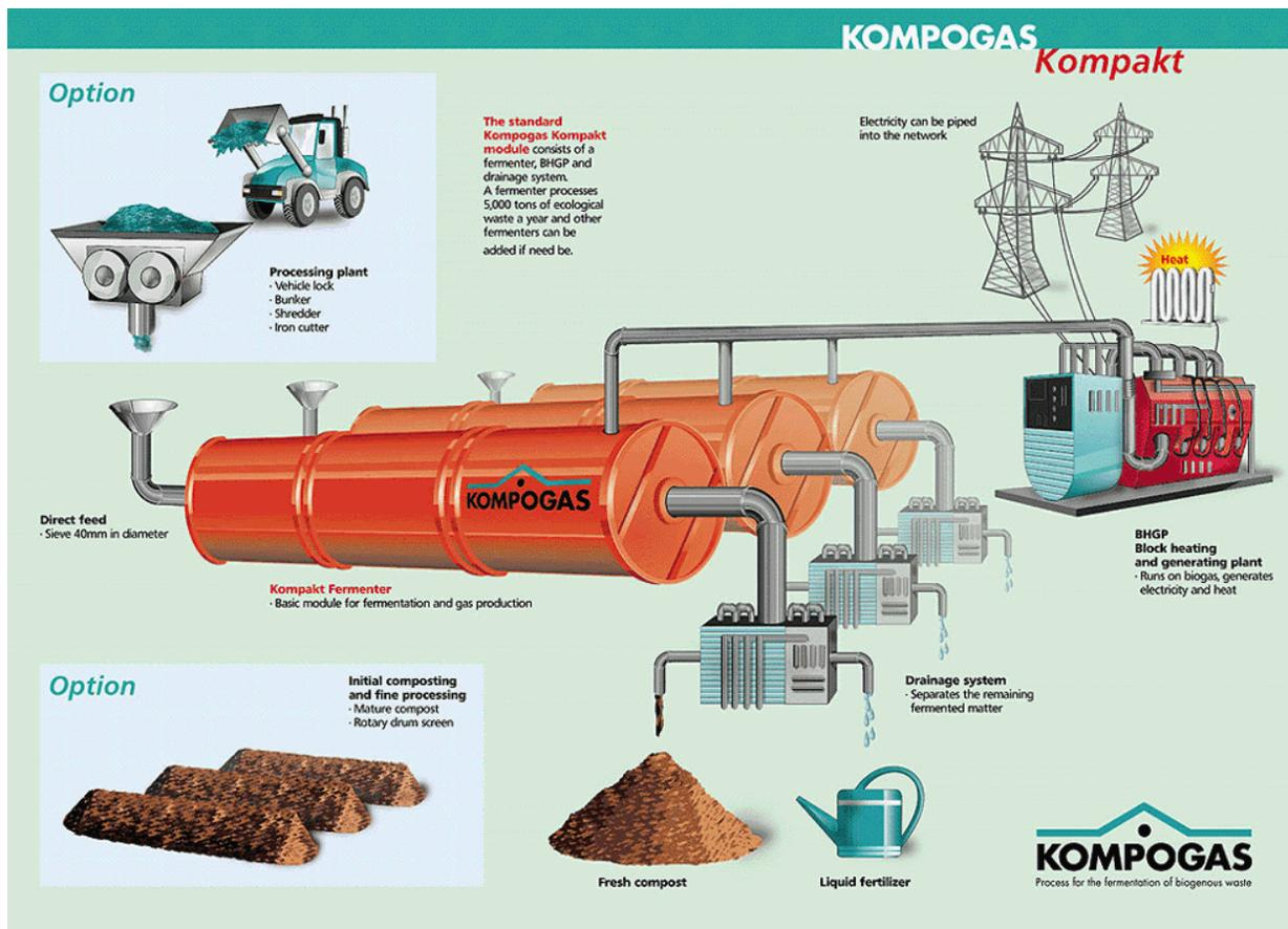
**Figure 15. Overview of the KompoGas process**
