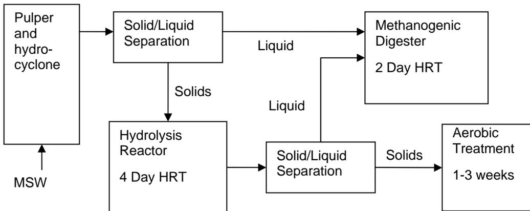
**Figure 17. Diagram of the BTA multistage digestion process**
