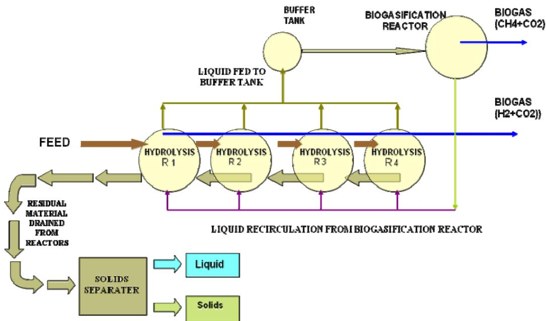
**Figure 23. Schematic diagram of the APS Digester system.**
