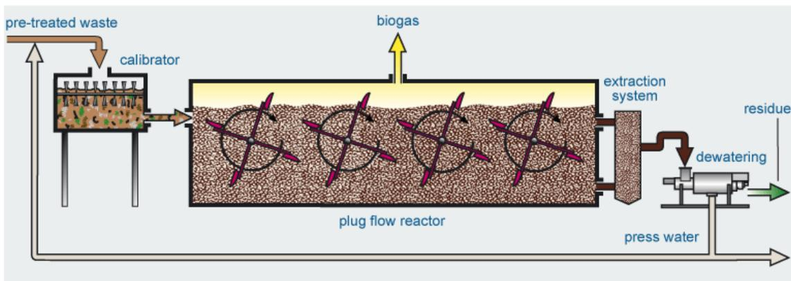
**Figure 18. Linde-KCA two-stage dry digester**
