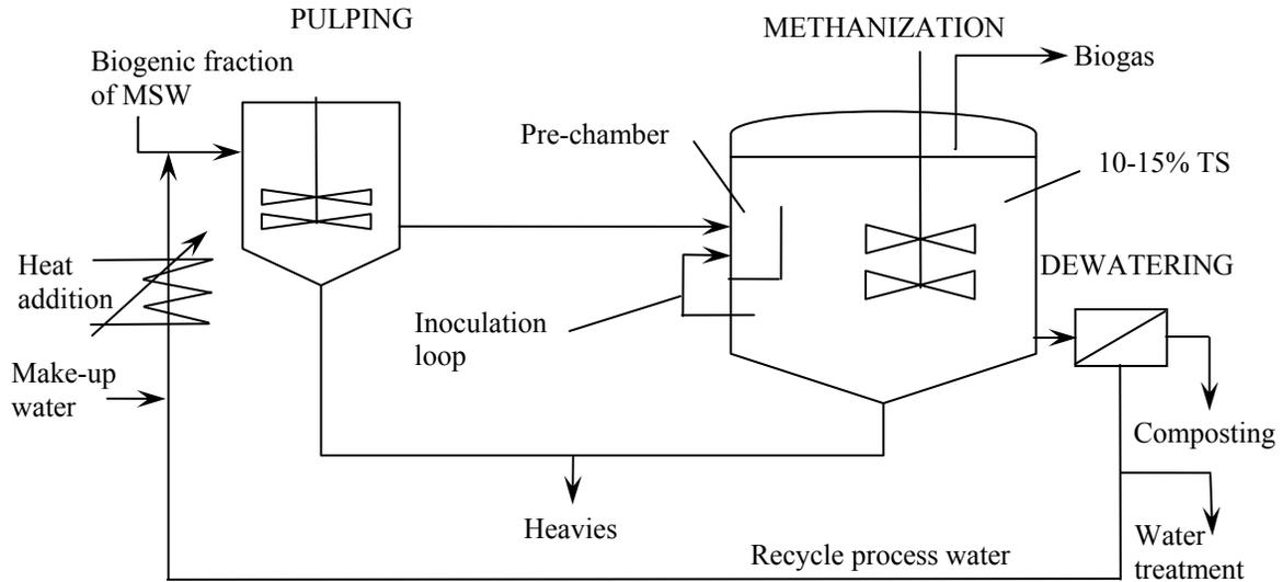
**Figure 10. Schematics of the Waasa one-stage digestion process [45].**
