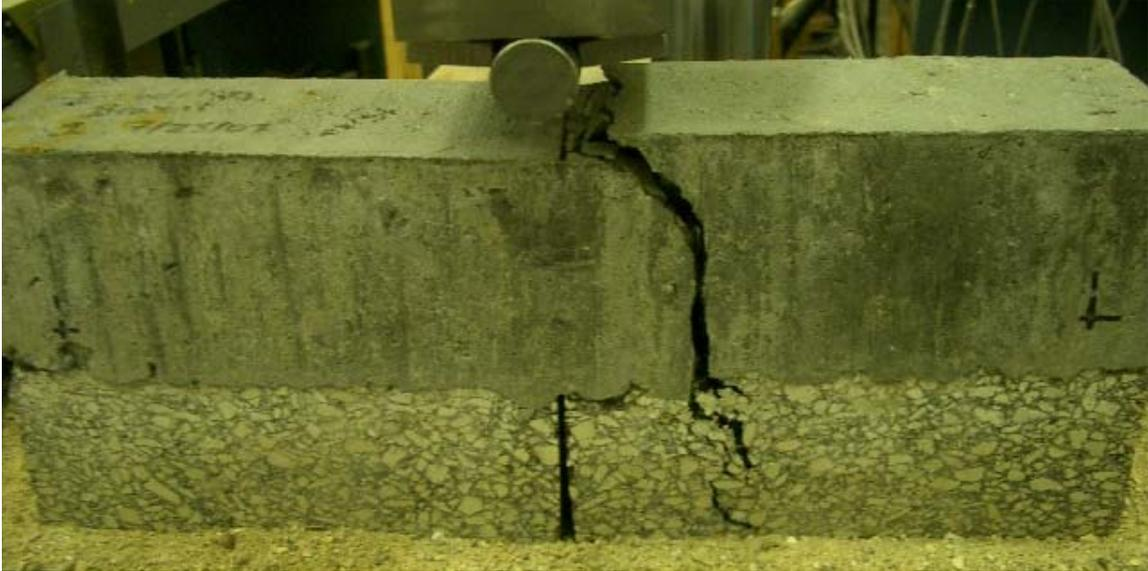
*Figure C.31. Failure pattern in the second Brazil 2 composite beam specimen.*
