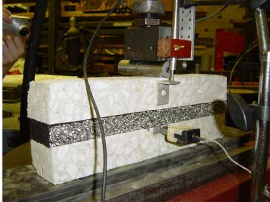
Figure C.20. Initial composite (concrete on concrete) test setup (from Braham 2006).
