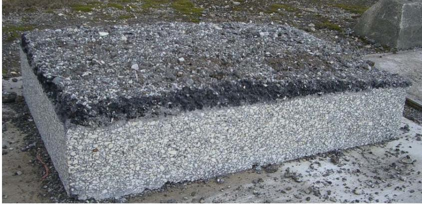
Figure C.32. Photo of an upside-down HMA section prior to saw-cutting into beam sizes.
