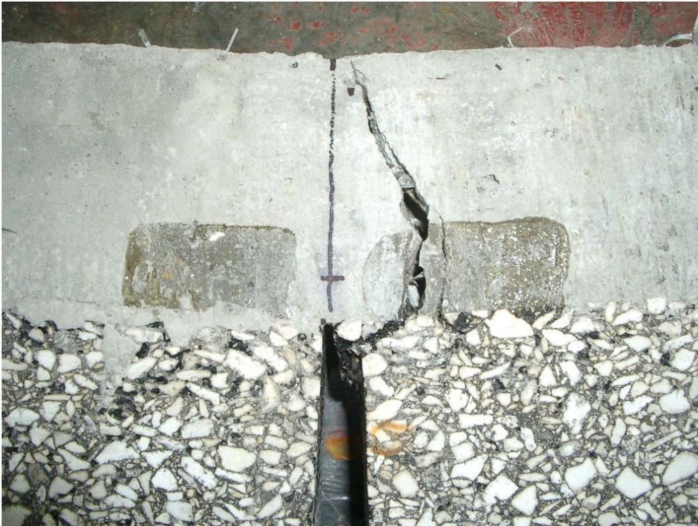
Figure C.30. Picture of fractured composite beam.
