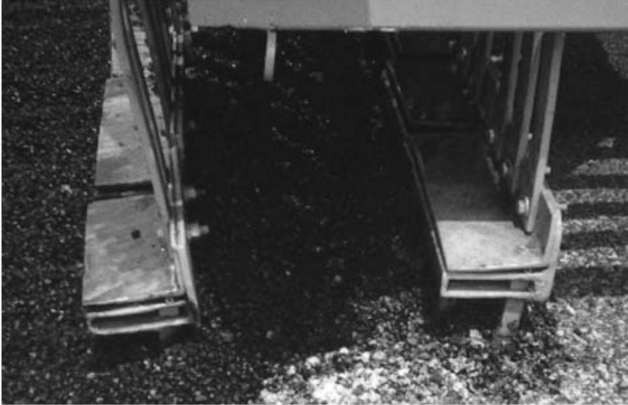
*Figure 1-8: Surface Recycling scarification teeth*
