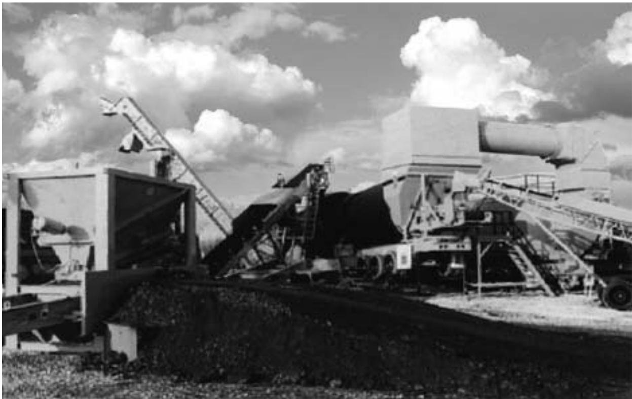
*Figure 1-6: Drum mix plant with RAP infeed for hot recycling*
