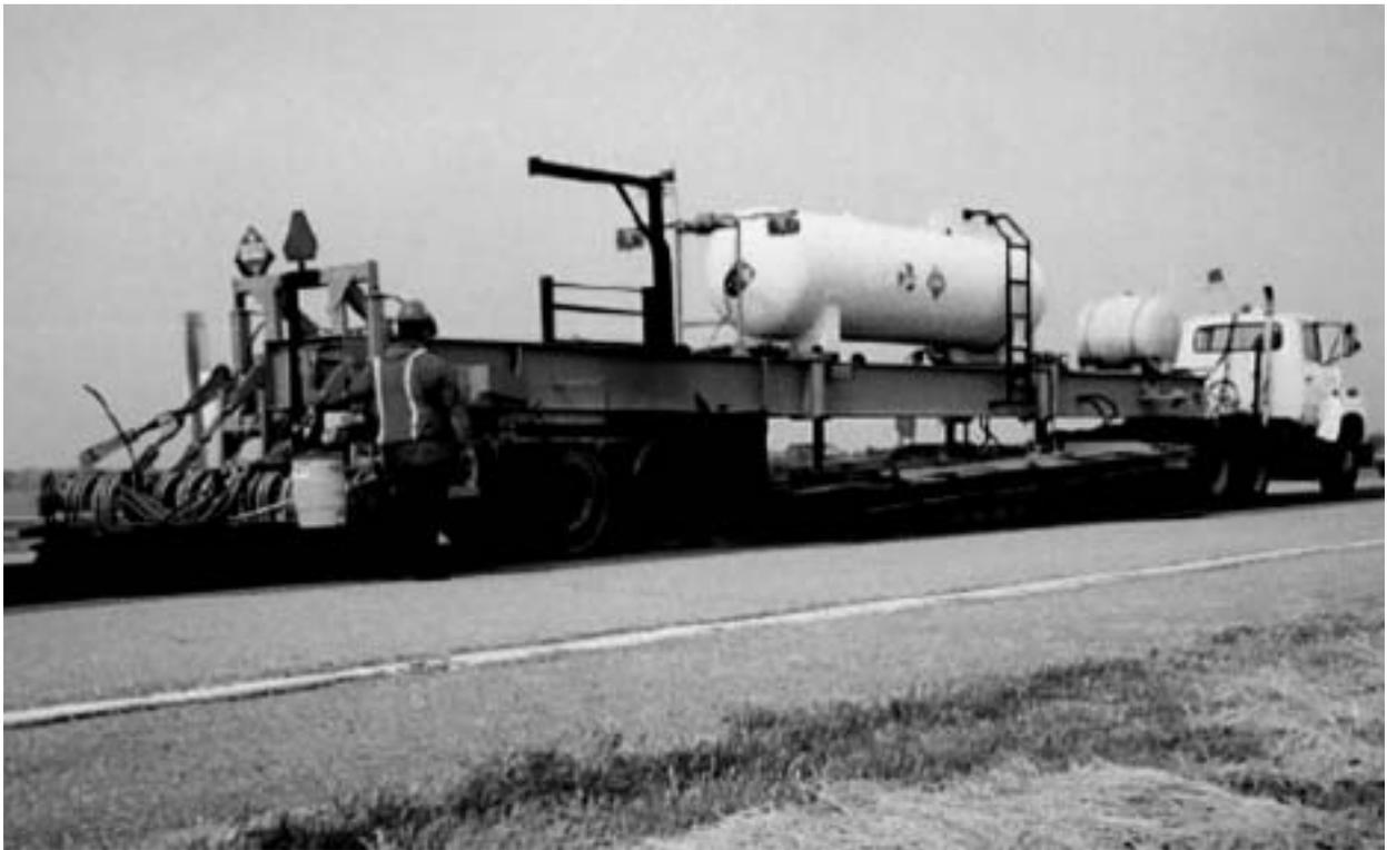
*Figure 6-2: Heating and scarifying unit*
