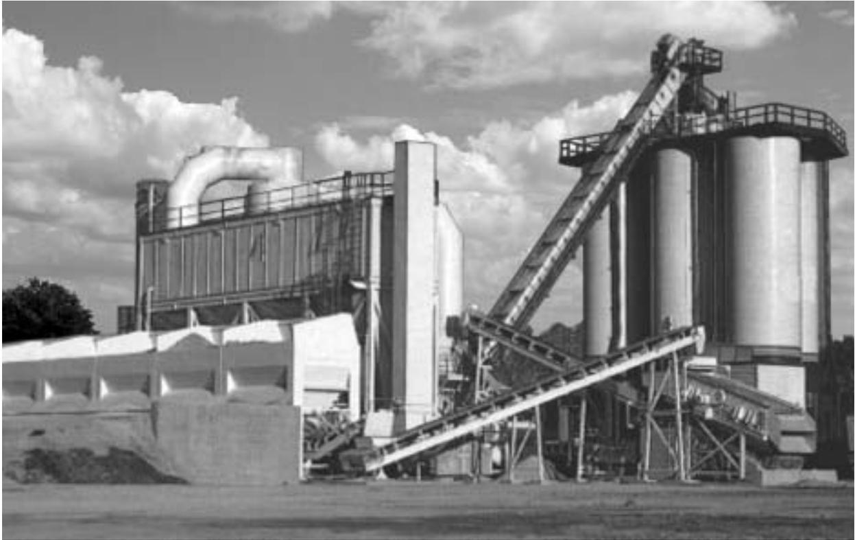
*Figure 1-5: Asphalt batch plant with RAP infeed for hot recycling*
