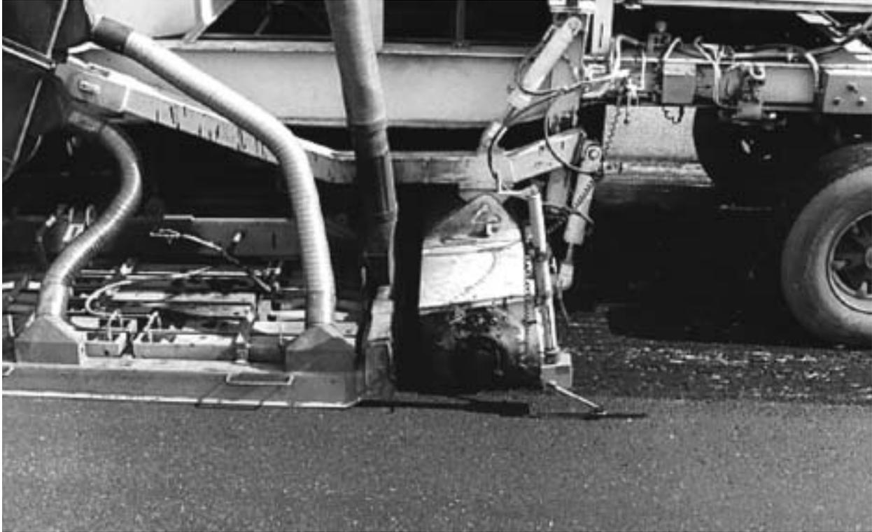
*Figure 6-13: Hot milling drum and matching shoe*
