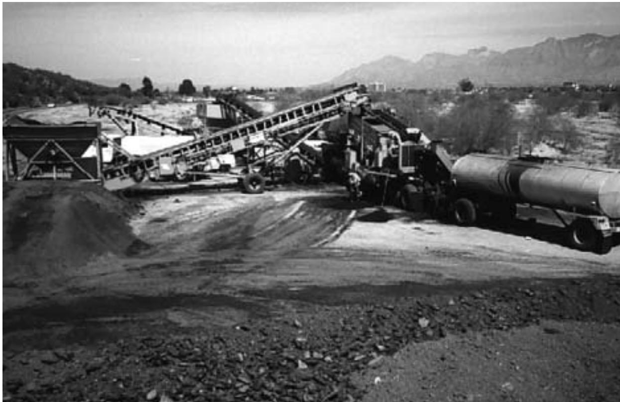
*Figure 1-23: CIR train set up as a stationary plant*
