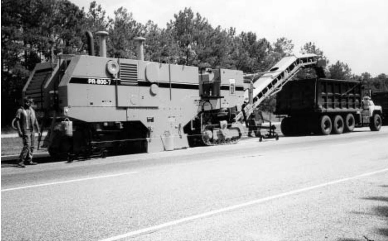
*Figure 1-2: Typical front loading milling machine*
