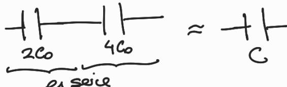
$$\frac{1}{C} = \frac{1}{2C_0} + \frac{1}{4C_0} = \frac{1}{2C_0} \left(1 + \frac{1}{2}\right) = \frac{3}{4C_0} \Rightarrow C = \frac{4C_0}{3}$$
