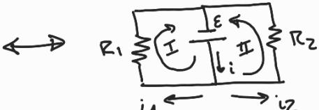
$$\text{De (2)} \quad E = BlN_A \quad \left| \begin{array}{l} \rightarrow \text{de (I): } i_1 = \frac{E}{R_1} = \frac{BlN_A}{R_1} \\ \rightarrow \text{de (II): } i_2 = \frac{E}{R_2} = \frac{BlN_A}{R_2} \end{array} \right.$$
