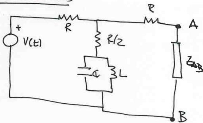
$$\bar{V}(t) = V_0 e^{j\omega t}$$
