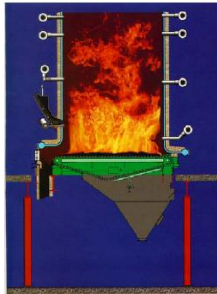
Figure 4 – Air-Cooled Travel Grate
